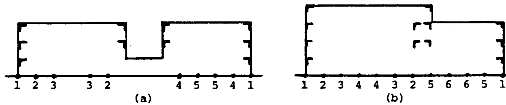
Figure IV.18: Problems with marker tracing: gaps (a) and domination (b).
