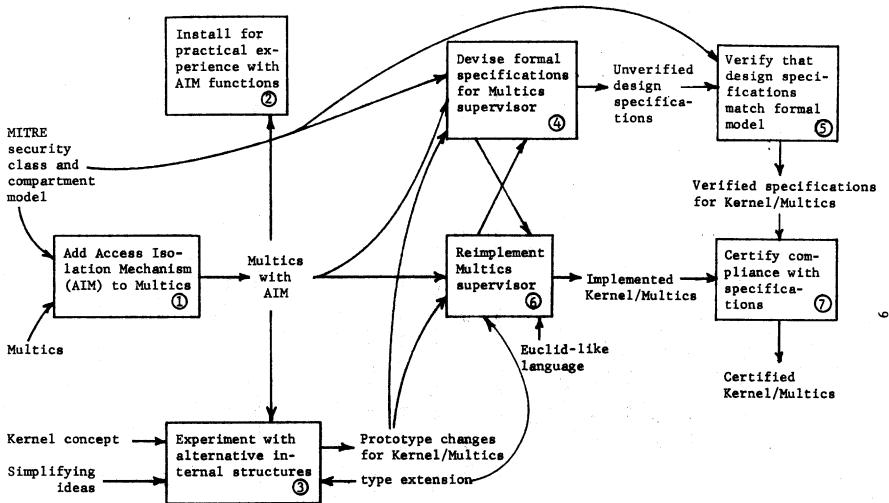
Figure 1 -- Plan for developing a certifiable security kernel for Multics
