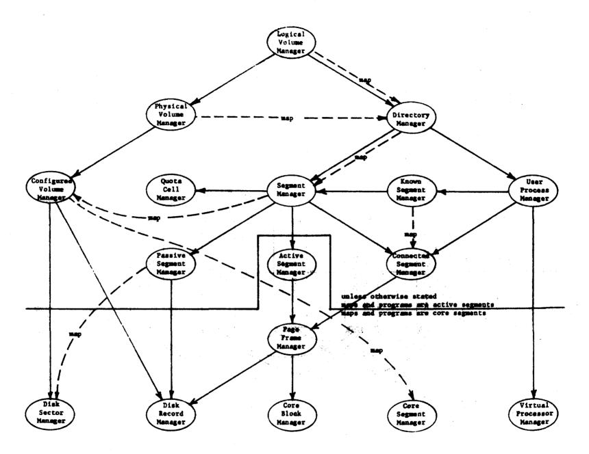
interpreter dependencies: every module, except the Core Segment Manager, depends on the Virtual Processor Manager address space dependencies: every module, except the Core Segment Manager, depends on the Core Segment Manager
