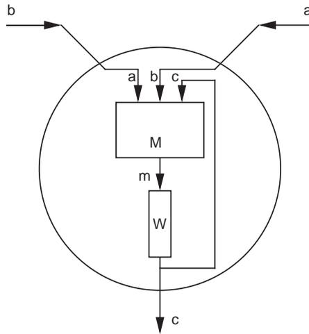
Figure 2: A majority element and a wire implementing a Muller C element
