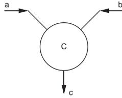
Figure 1: The Muller C element
