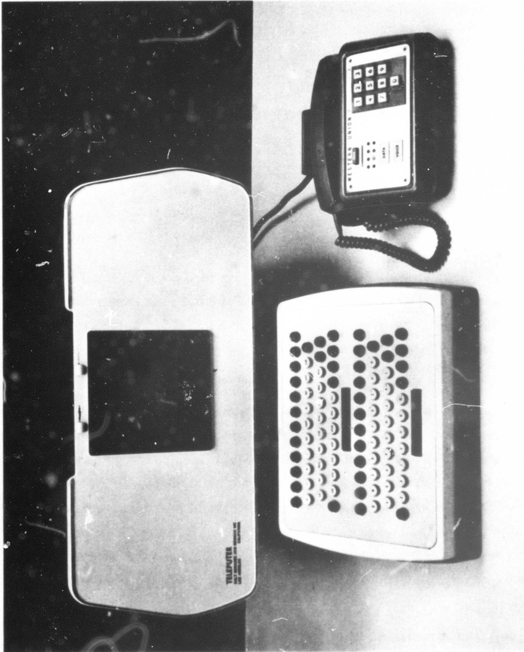
Figure 27. Project TACT Remote Culler-Fried Display Terminal
