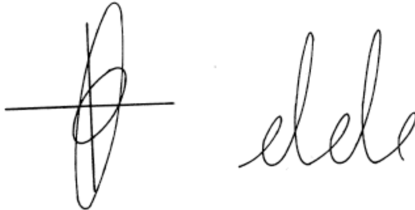
Figure 2.5. Modulation of the vertical oscillation at points of zero vertical velocity yields different letter heights by a process of amplitude modulation without phase change.
