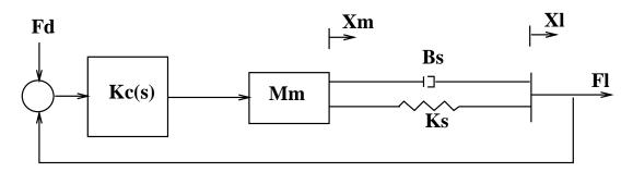
Figure 6-1: Series elastic actuator model. Mm is the motor mass. Ks and Bs are the spring constant and damping constant. Kc(s) is the compensator. Fd is the desired force while Fl is the actual force applied to the load. Xm and Xl are the motor and load displacements.
