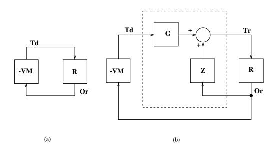
Figure 6-2: Block diagrams of a) Virtual Model (VM) and Robot (R) with perfect torque controllers and b) with non-ideal controllers. G is the torque controller transfer function matrix and Z is the torque controller impedance matrix.
