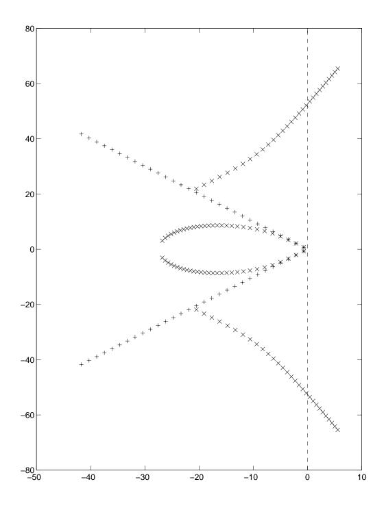
Figure 8-4: Locus of closed loop poles as  $\omega_v$  is increased from 1 to 60. At low  $\omega_v$ , the poles due to desired dynamics dominate. At high  $\omega_v$ , the poles due to the actuator dynamics dominate and eventually enter the right half plane.
