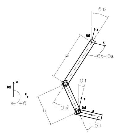
Figure 3-3: Foot example.  $\theta_t$  is the toe angle,  $\theta_a$  is the ankle angle,  $\theta_f$  is the angle of the foot with respect to frame {O}, and  $\theta_b$  is the angle of the body with respect to frame {O}.
