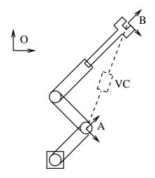
Figure 2-1: Virtual Component Reference Frames.  $\{B\}$  is the action frame.  $\{A\}$  is the reaction frame.  $\{O\}$  is the reference frame. VC represents the virtual component. The virtual component is drawn schematically to show it acts between frames  $\{A\}$  and  $\{B\}$ . The forces exerted by the virtual component can be in any admissible direction.
