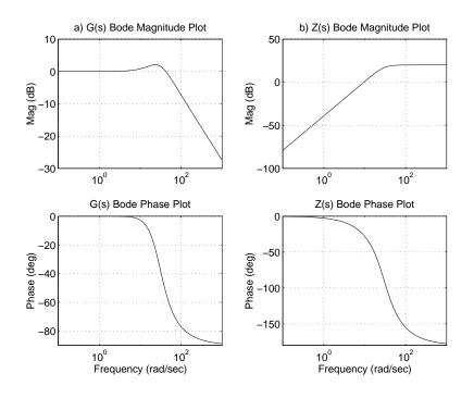
Figure 6-3: Typical bode diagrams of G(s) and Z(s) for Series Elastic Actuation. Ideally G(s) = 1(0 db Gain, 0 deg Phase) and Z(s) = 0 (-  $\infty$  Gain, 0 deg Phase). This is a good approximation at low frequencies but poor at high frequencies. At high frequencies  $G(s) \approx 0$  and  $Z(s) \approx K_s$ .
