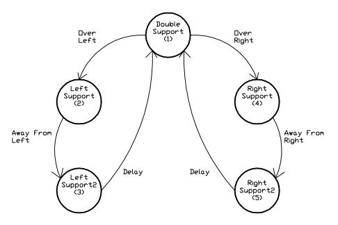
Figure 9-4: State machine used in the Stupid Walking algorithm.
