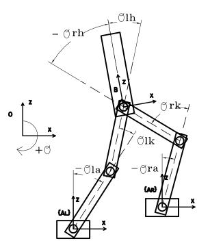
Figure 3-2: Dual Leg example. Reaction frames {A} and {C} are assumed to be in the same orientation as reference frame {O} so that  ${}^{O}_{A_{I}}R = {}^{O}_{A_{r}}R = I$ .
