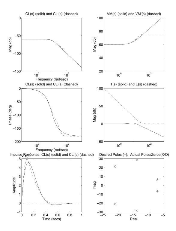
Figure 8-2: Simple SISO example with  $\omega_v = 10.0$
