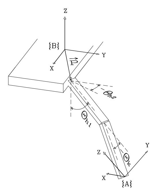
Figure 3-5: Diagram of a single leg of the hexapod example. There is one actuated degree of freedom at the knee and two at the hip. The knee angle is  $\theta_k$  and the hip angles are  $\theta_{h1}$  and  $\theta_{h2}$ . The leg links are both of length L. The location of the leg with respect to frame {B} is  $(P_x, P_y, 0)$ .
