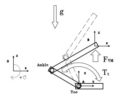
Figure 4-1: Simple foot example showing virtual model forces,  $F_{VM}$  and required to torque,  $T_t$ .
