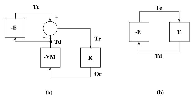
Figure 7-1: a) Virtual model error expressed as a multiplicative error (E). b) VM and R are combined into T for the linear case so that the Small Gain Theorem can be employed.
