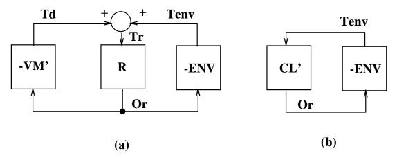
Figure 7-3: Robot (R) and virtual model controller (VM') as seen by the environment (ENV). In b) CL' is the closed loop admittance of the system as seen by the environment.
