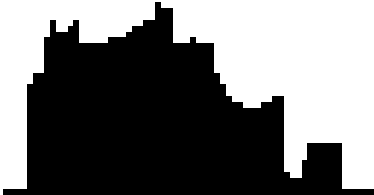
Figure 1.4: The set of textureless pixels corresponding to the carpet. Note that the blob is taller where there is more exposed carpet.
