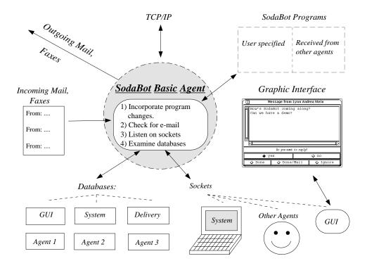
Figure 2-1: The SodaBot basic software agent architecture
