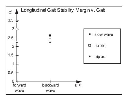
Figure 4.27: Hannibal's gait stability margin for various gaits.
