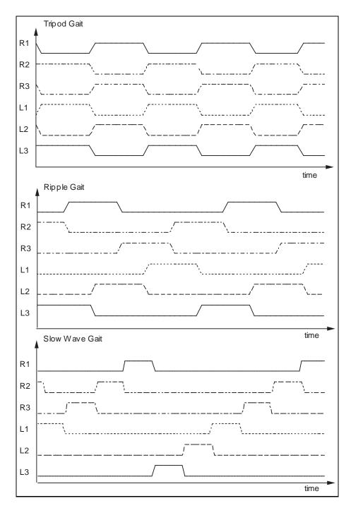
Figure 4.20: Run-time data of various gaits implemented on Hannibal using the pacemaker scheme.
