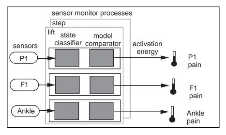
Figure 6.6: The sensor monitor processes for the ground-contact virtual sensor and step-in-hole virtual sensor.
