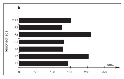
Figure 4.31: Time taken to walk three feet with various legs disabled.
