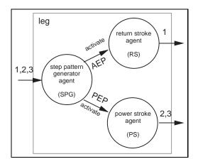
Figure 4.8: The cyclic stepping pattern of each leg was implemented using this circuit. The step pattern generator agent produced the step cycle by exciting the return stroke agent and the power stroke agent in turn. The arrows with numbers represent the direction the coordination mechanisms were sent between the legs. The numbers represent Cruse's coordination influences as labeled in this section.
