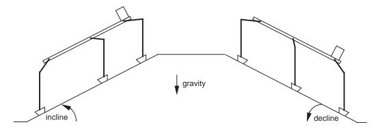
Figure 5.9: Hannibal servos its spine motor to keep its legs vertical when walking over undulating terrain. This maintains the robot's stability by keeping its center of mass withing the polygon of support.
