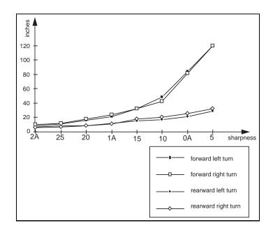
Figure 4.29: Relation of turn sharpness to sharpness parameter.
