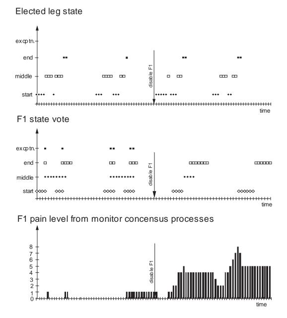
Figure 6.9: Response of the monitor consensus processes to vertical force sensor failure. Once the sensor fails, it disagrees frequently with the complementary sensors. Consequently, the sensor's pain level increases .
