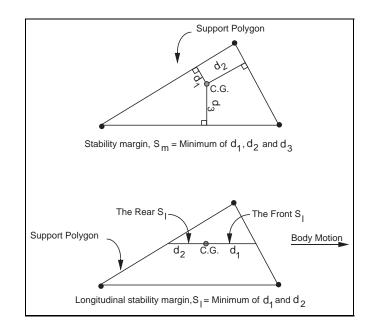
Figure 4.26: Graphical depiction of the stability margin and longitudinal stability margin.
