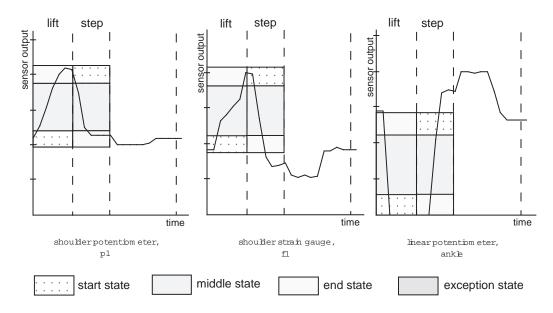
Figure 6.5: The relationship of sensor output to step cycle phase and leg state for the sensors used by the ground-contact virtual sensor.
