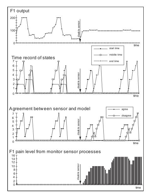
Figure 6.7: Response of the sensor monitor processes to vertical force sensor failure. Once the sensor fails, the actual sensor behavior frequently disagrees with the modeled sensor behavior. Consequently, the sensor's pain level increases.
