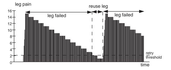
Figure 6.24: The system occasionally retries to use the leg. If it works again, the system reincorporates the use of that leg.
