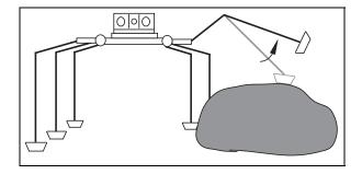
Figure 5.8: When the robot's foot is stepping on a medium sized obstacle, the foot needs to be lifted higher during the recover phase. Otherwise, the foot will drag along the top of the obstacle as the robot swings the leg forward.
