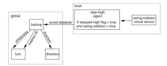
Figure 5.11: This network causes the robot to back away from obstacles that are too large to step over. The backup agent is activated when a leg collides with and obstacle after its foot is lifted as high as possible off of the ground. The global backup agent sets the number of steps the robot walks backwards and the turn sharpness based on the avoid-obstacle message. The direction of rotation is set such that the robot turns away from the obstacle.
