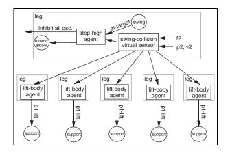
Figure 5.6: For each leg, the step-high agent is activated when the output of the swing-collision virtual sensor is **true**. When active, the step-high agent causes the foot to rise off the ground by activating the extend-elbow agent. Once the elbow is fully extended, the leg swings to its target value. The swing agent de-activates the step-high agent when the leg reaches the target value. Once this occurs, the elbow is contracted and the leg steps down.
