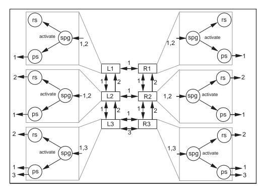
Figure 4.11: The Modified Cruse Control gait coordination circuit.
