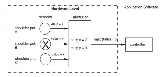
Figure 6.2: Replication of components is often used at the hardware level to make the system tolerant of hardware failures.
