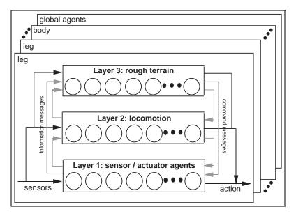
Figure 3.2: Hannibal's control task is distributed among several subsumption-based controllers.
