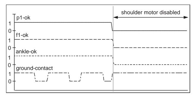
Figure 6.21: If the shoulder actuator fails, the ground-contact virtual sensor masks its output from the high level control.
