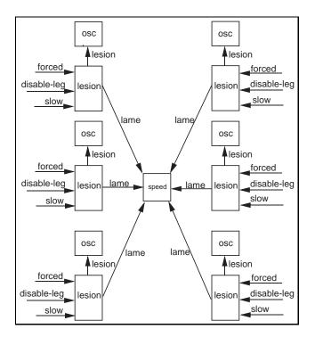
Figure 4.25: This network enables the robot to walk in a stable fashion despite leg damage. When the lesion agent of a leg is active, the lesion agent sends a message to the global speed behavior to make the robot adopt the slow wave gait. This gait is stable even with fewer than six legs are working. In addition, the lesion agent places the motors of its leg in brake-mode and removes the influences of its from the rest of the network.
