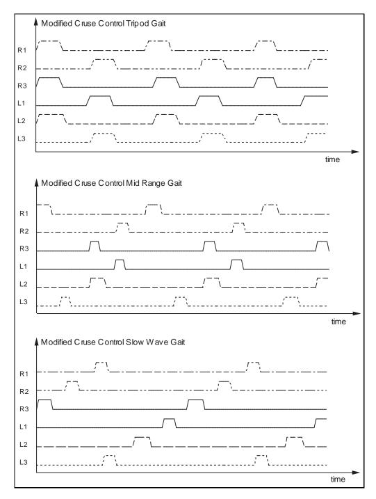
Figure 4.13: Various gaits produced using Modified Cruse Control.
