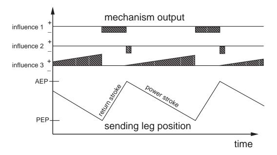
Figure 4.7: Relation of the coordinating mechanisms to leg position.
