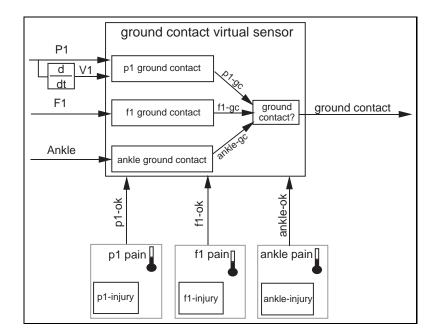
Figure 6.12: Illustration of a robust ground-contact virtual sensor.
