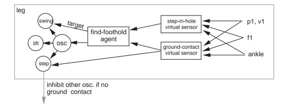
Figure 5.5: For each leg, the find-foothold agent is activated once the output of the step-in-hole virtual sensor is **true**. While active, it generates the searching pattern by making the leg's oscillator agent repeat the recover phase with new target values. Meanwhile, the leg's step agent makes the robot pause by inhibiting the oscillators of the supporting legs. The findfoothold agent is de-activated when the output of the ground-contact virtual sensor is **true**.
