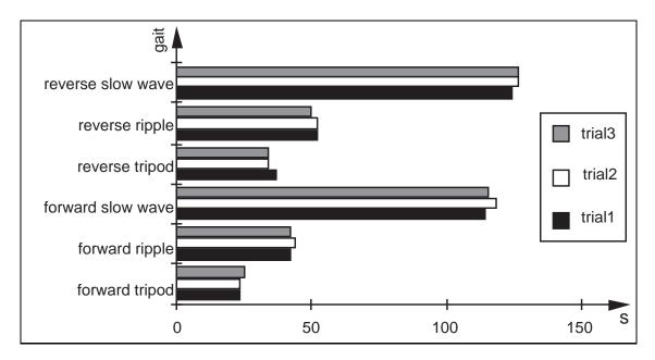
Figure 4.30: Comparison of times required to walk three feet either backwards or forwards.
