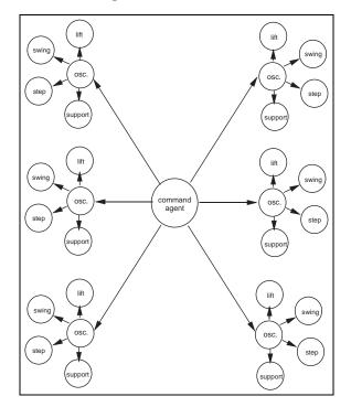
Figure 4.17: Gait coordination circuit for the pacemaker scheme. This circuit is strongly inspired by the work of Pearson.
