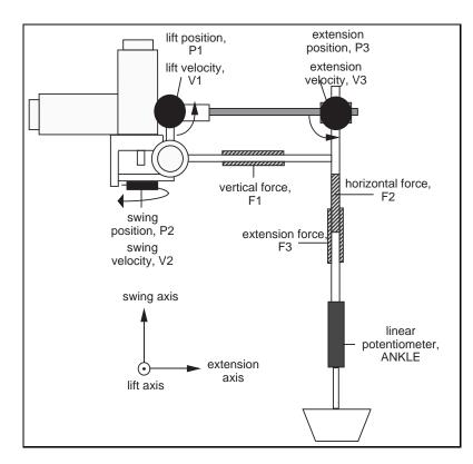
Figure 2.3: Leg mounted sensors with labels.
