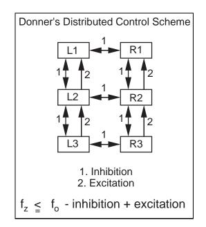
Figure 4.33: Locomotion controller for the SSA Hexapod. Adapted from (Donner 1987).
