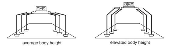
Figure 5.7: The robot's body can be elevated by activating the lift-body agents of the supporting legs. For example, when the output of a leg's swing-collision virtual sensor is **true**, the swing-collision virtual sensor activates the lift-body agents of the supporting legs. This helps the collided leg clear the obstacle.
