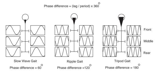
Figure 4.4: Various gaits emerge from changing the frequency of the local leg oscillators.
