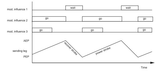
Figure 4.12: The influences used in the Modified Cruse Control gait coordination mechanism.
