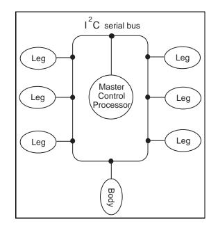
Figure 2.4: Hannibal's smart subsystems are linked by a serial network.
