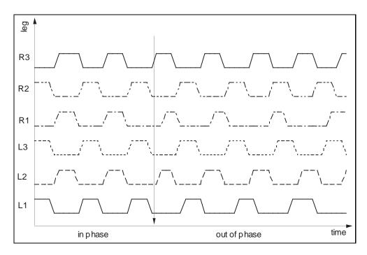
Figure 4.10: After implementing Cruse Control on Hannibal, we found that insufficient velocity control of the legs caused the gaits to shift in and out of phase.
