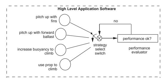
Figure 6.3: Robust behavior can be implemented using redundant strategies.
