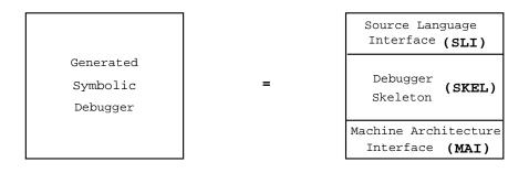
Hgure 1-2: The Components of a Generated Debugger
