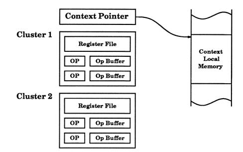
Figure 5.7: The state associated with a thread. This thread is for a machine with two clusters, each with two function units. The thread has a register file in each cluster and an Operation Pointer (OP) and Operation Buffer in each function unit. The Context Pointer (CP) points to the thread's local memory.
