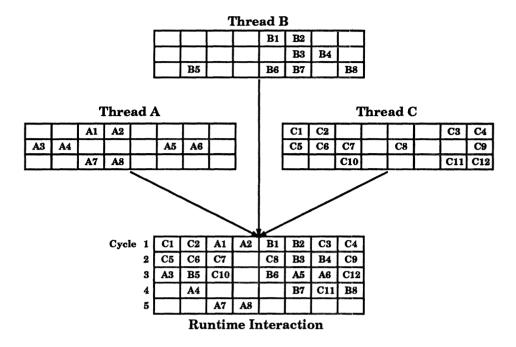
Figure 1.1: Interleaving of instruction streams. Threads A, B, and C are scheduled separately and their instruction streams are shown at the top of the diagram. Each column is a field for a particular function unit and each row holds those operations which are allowed to execute simultaneously. The bottom box shows a runtime interleaving of these threads in which some operations are delayed due to function unit conflicts.
