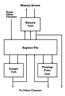
Figure 3.2: The prototypical cluster contains three function units: a memory unit, an integer arithmetic unit, and a floating point unit. Each share access to a common register file. The memory unit communicates with the memory system. Each unit can send its results to the local register file as well as to the register files of remote clusters.
