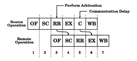
Figure 7.4: Bypassing data from the EX stage of a source unit to the EX stage of a remote unit. Arbitration for communication resources is performed during the RR stage. The single cycle communication latency delays the result from arriving at the destination until cycle 6.
