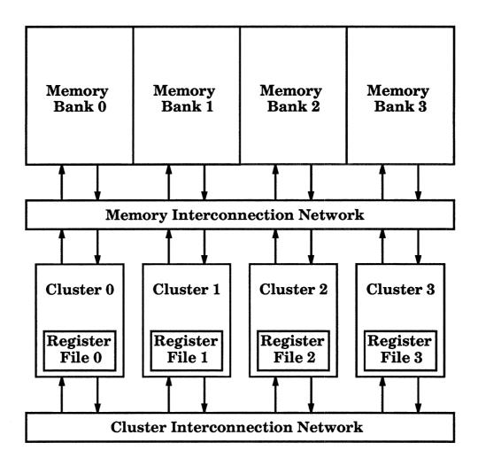
Figure 3.1: This sample machine consists of four clusters, each of which contains a register file and some number of function units. The clusters communicate with each other through the Cluster Interconnection Network and through memory.
