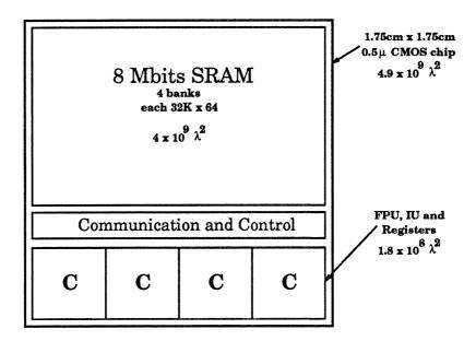
Figure 7.6: Floorplan for a four cluster multi-ALU processing node.
