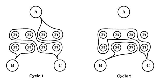
Figure 1.2: Two possible mappings of function units to threads. These mappings correspond to the first two cycles shown in Figure 1.1.
