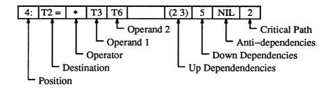
Figure 4.7: Three address code statuent computing  $T3 \times T6 = T2$ .
