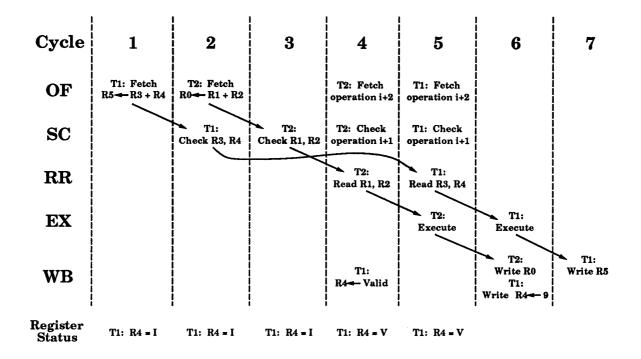
Figure 7.2: The procession through the pipeline of operations from two different threads (T1 and T2). T1's operation is fetched during cycle 1, and during cycle 2 it checks the scoreboard and finds R4 invalid. T2's operation is fetched in cycle 2, checks the scoreboard during the cycle 3, and since both source registers are valid, issues to the RR stage during cycle 4. T1's register R4 becomes valid at the end of cycle 4 and it follows T2's operation into the RR stage in cycle 5.
