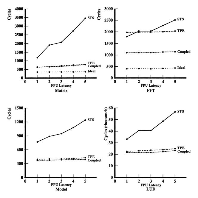
Figure 6.5: Cycle counts when floating point unit latency is varied.
