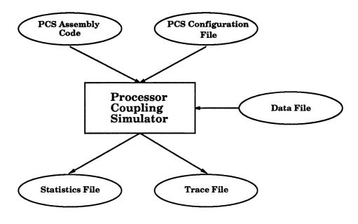
Figure 5.1: Simulator inputs and outputs.
