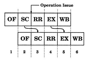
Figure 7.3: A five stage pipeline corresponding to the function unit in Figure 7.1. The first operation updates the scoreboard as it issues to the RR stage, two cycles before the result is ready. The next operation can issue immediately and use the bypassed result from the EX stage.
