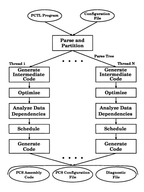
Figure 4.5: Compiler flow of control. The program and configuration files are used by the parser and partitioner which generate intermediate code. Each thread has its own intermediate code which proceeds through the optimization, data dependency analysis, scheduling, and code generation stages. The output is a new configuration file, the assembly code, and a diagnostic file.
