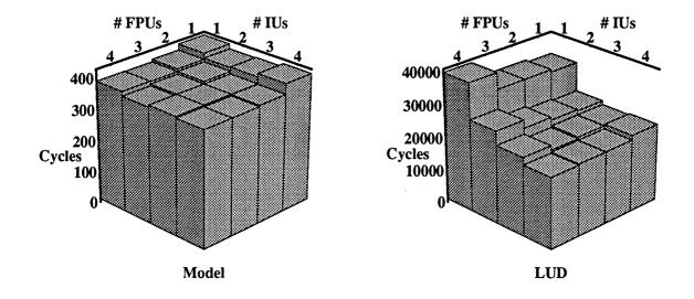
Figure 6.7: Cycle count as a function of number of Floating Point Units (FPUs) and Integer Units (IUs). For a fixed number of function units, cycle count is minimized when equal numbers of IUs and FPUs are used.
