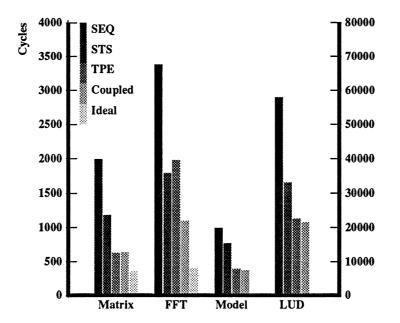
Figure 6.2: Baseline cycle counts for the five simulation modes. Matrix, FFT, and Model, are referenced to the left axis, while the scale for LUD is on the right. Ideal is only implemented for Matrix and FFT.
