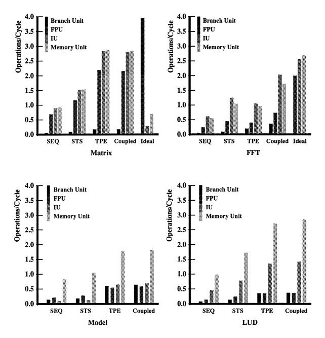
Figure 6.3: Function unit utilization.
