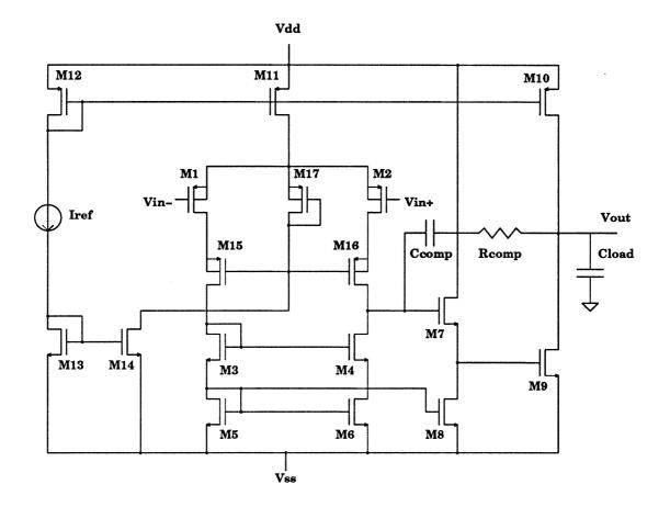
Figure 6.1: Operational Amplifier circuit used in the model evaluation benchmark.
