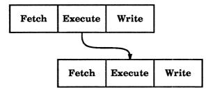
Figure 5.4: The simulator function unit pipeline has three stages. The Fetch and Write stages are one cycle each. The Execute stage shown is one cycle but it can be specified by the user. Results are bypassed from one Execute stage to the next so that one thread can issue an operation on every cycle.
