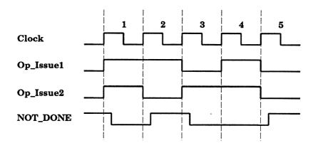
Figure 7.5: The NOT\_DONE signal indicates when all of the operations scheduled in an instruction have been issued. The **op\_issue** waveforms are asserted when an operation issues from the SC stage to the RR stage. NOT\_DONE remains asserted until both operation 1 and operation 2 have issued.
