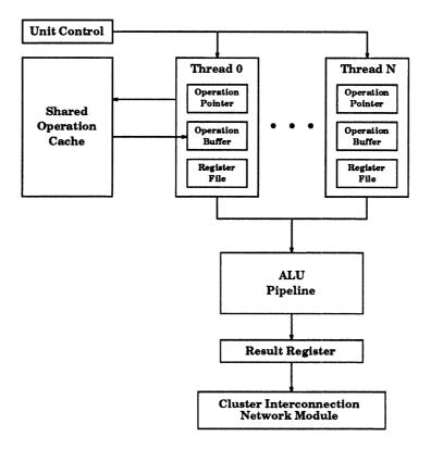
Figure 5.5: Simulator function unit model. Each function unit has an operation pointer and an operation buffer for each thread. The register file for a thread is shared with other function units in the cluster. The operation cache is shared by all active threads.
