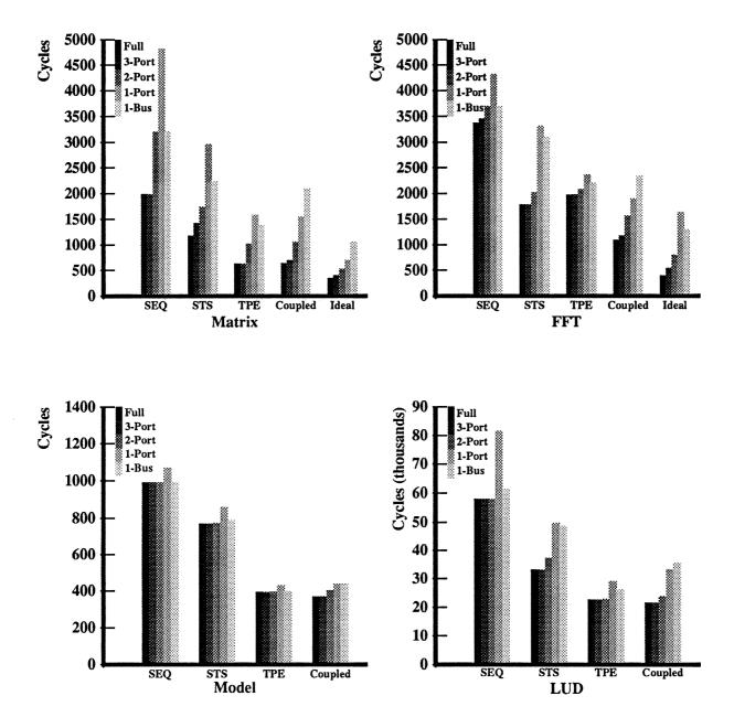
Figure 6.6: Cycle counts for restricted communication schemes of Processor Coupling. Cycle count increases dramatically when single buses and ports are used, but the Tri-Port scheme is nearly as effective as the fully connected configuration.
