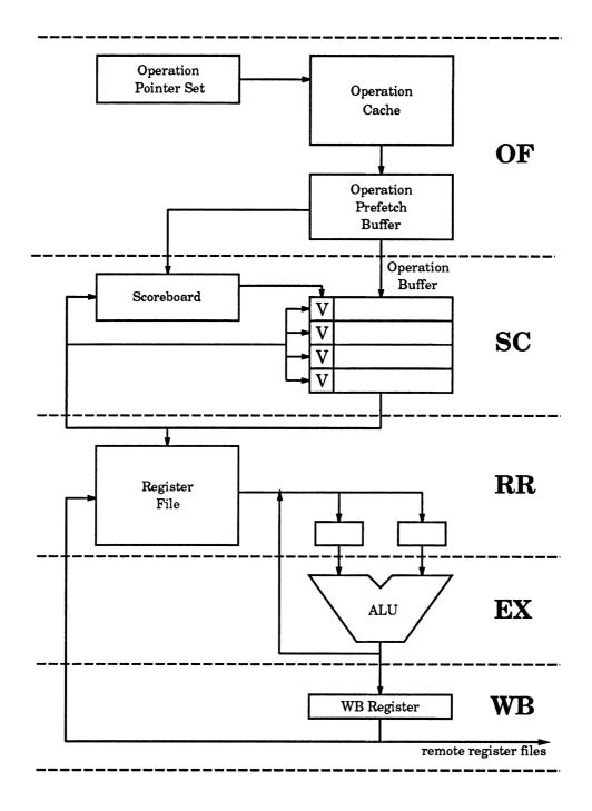
Figure 7.1: A sample arithmetic unit with a single EX stage. OF fetches an operation from the Operation Cache, SC checks the scoreboard to determine which of the source registers are ready, RR reads the register file, EX executes the operation, and WB writes back the result.
