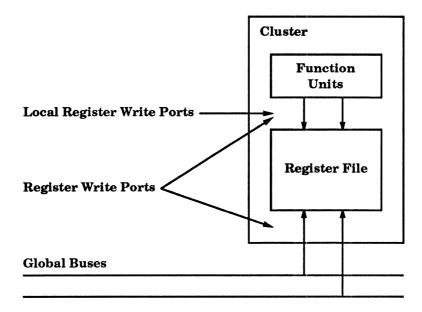
Figure 5.6: Interconnection network buses and ports. Writes to the local register file can use any of the register file ports. Remote writes may not use the local register write ports.
