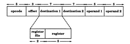
Figure 3.5: This operation devotes 5 bits to the opcode and 3 bits to the offset for the next executable operation. Destinations are specified using 2 bits to identify the cluster and 5 bits to identify the register. The two source registers are specified using 5 bits each.
