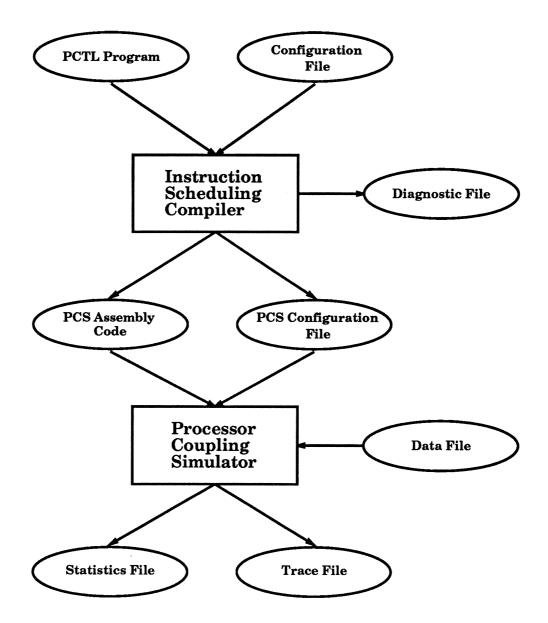
Figure 4.1: The flow through the simulation environment. PCTL programs are compiled into PCS assembly code by the Instruction Scheduling Compiler (ISC). PCS runs the program using the input data provided by the Data File. ISC determines the machine parameters from the Configuration File and produces a modified PCS Configuration File for the simulator.
