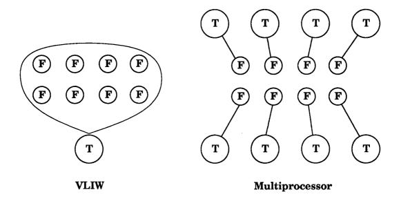
Figure 1.3: In a VLIW machine all of the function units are used by a single thread. The compiler uses as many units as it can and does not share them with other threads. In a purely multiprocessor organization, different threads run on different processing units and cannot couple multiple units together.
