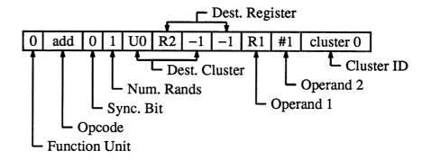
Figure 4.9: The fields of a PCS assembly operation.
