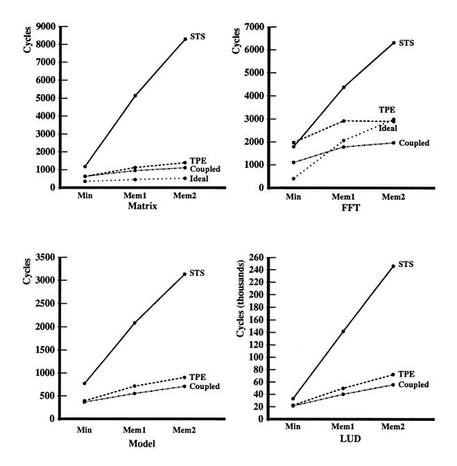
Figure 6.4: Cycle counts when memory latency is varied. Increased latency affects the single-threaded modes (STS and Ideal) more than the multithreaded modes (Coupled and TPE).
