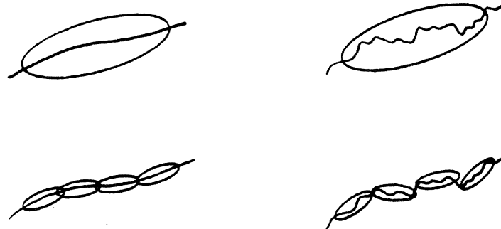
Figure 4.15: At coarse scales a long smooth edge and a long jagged edge appear identical. Only at finer scales do edge primitives obtain sufficient resolution to distinguish smaller scale detail.
