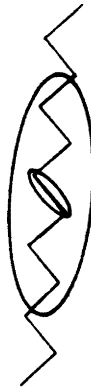
Figure 4.18: At a given spatial location, the jagged contour can give rise to edge primitives with different orientations at different scales.
