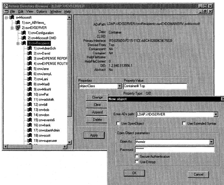
**Figure 15-16.** *The Active Directory Browser program. This program displays graphically the relationships and attributes of the objects contained in any directory that you can connect to using ADSI.*
