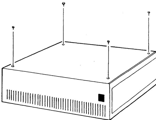
Fig. 10-1. Removing the  $\Omega$ 400 Top Cover
