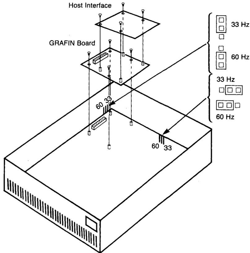
**Fig. 10-2. Location of Display Mode Jumpers**
