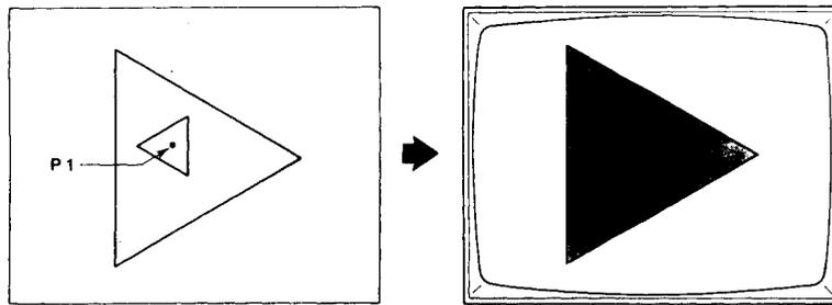
**Fig. 5-3. Outer Boundary Color Specified**
