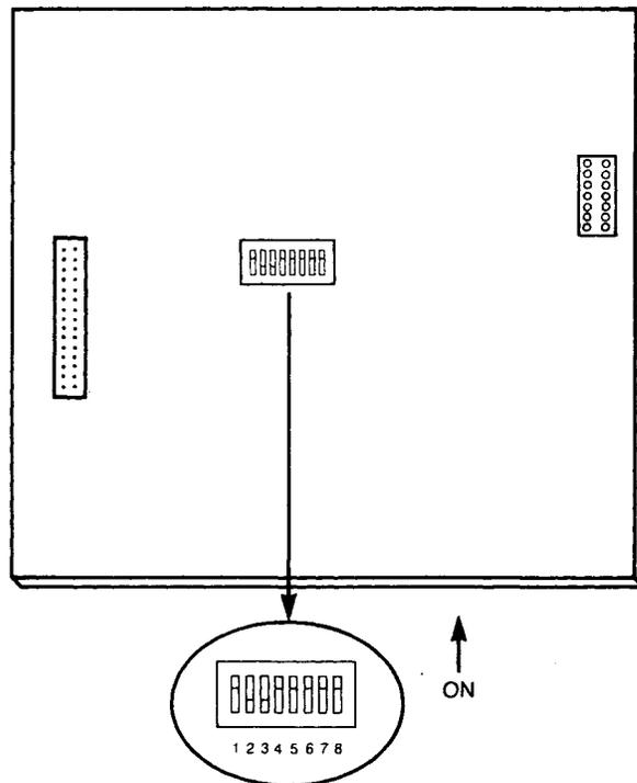
Fig. 10-3. Location of GRAFIN Data Transfer Rate Switches
