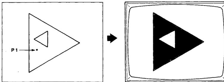
**Fig. 5-2. P1 set between boundaries of two different colors**
