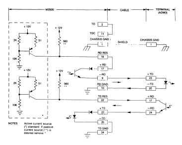
Figure 2-4: TTY Terminal Connector — Model 2500 Sources Current
