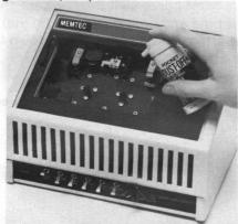
Figure 6-2: Preferred Cleaning of the EOT/BOT Sensor
