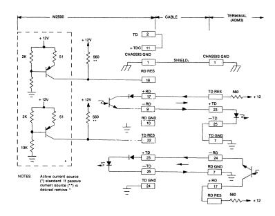
Figure 2-5: TTY Terminal Connector — Model 2500 Sinks Current
