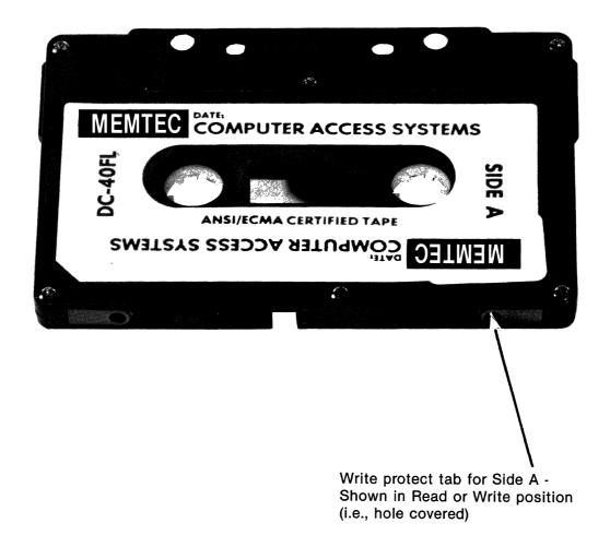
Figure 3-3: Movable Write-Protect Tabs
