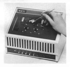
Figure 6-4: Cleaning the Recorder Head
