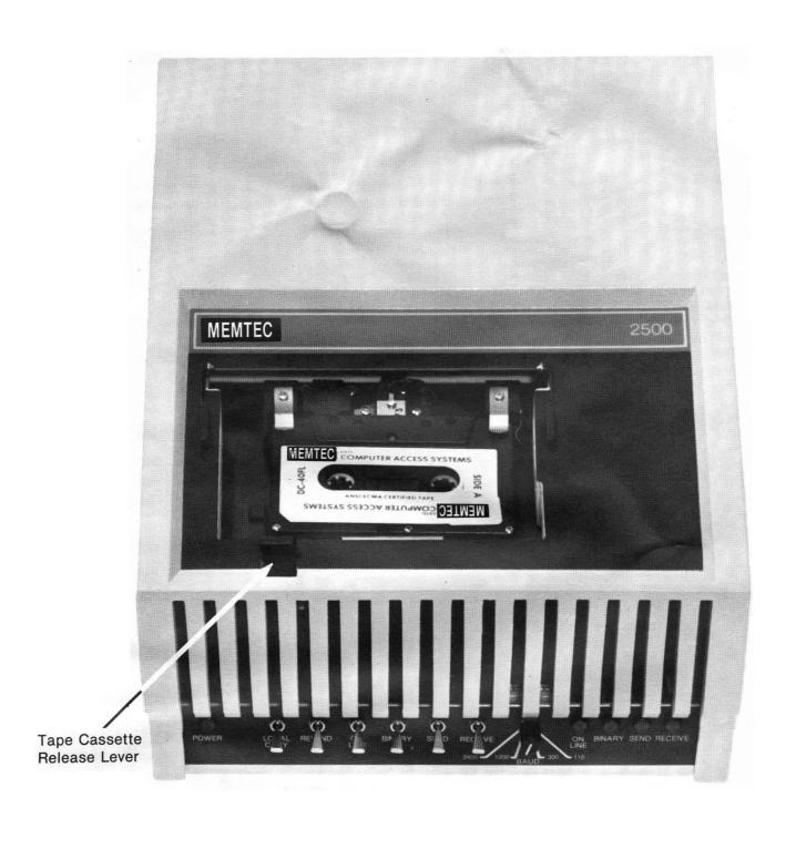
Figure 3-5: Tape Cassette Release Lever
