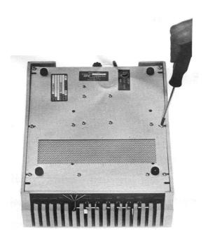
Figure 4-2: Removal of Captive Retaining Screws
