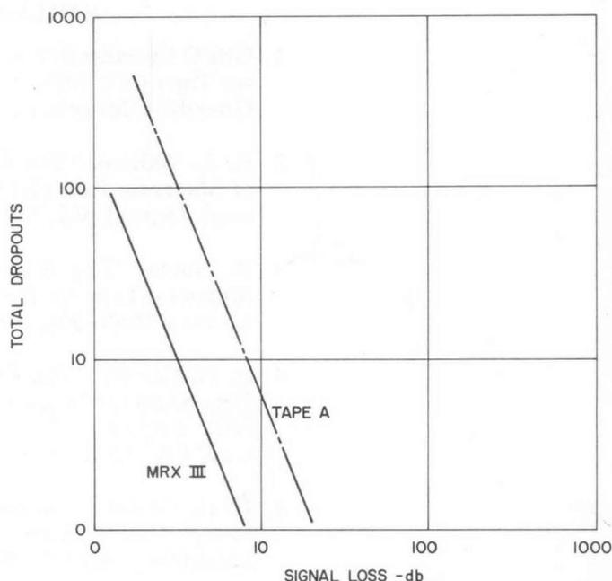
Figure 9. Total drop-outs as a function of detection level. As demonstrated by R. Noble's method of tape quality ranking. Drop-out distribution follows a power law.
