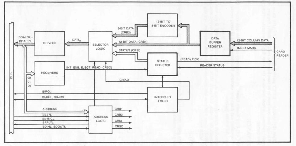
Figure 5. MLSI-CR11 Card Reader Controller, Simplified Block Diagram
