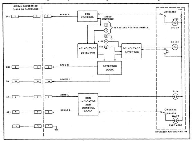
Figure 3-3 Power Sequencing Module, Simplified Block Diagram
