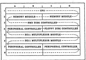
Figure 6-1 Recommended Module Placement
