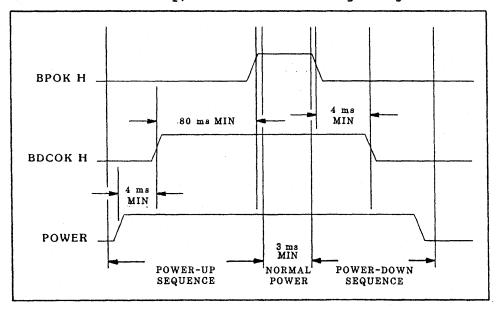
Figure 3-2 PSM Power-Up/Power-Down Timing Diagram
