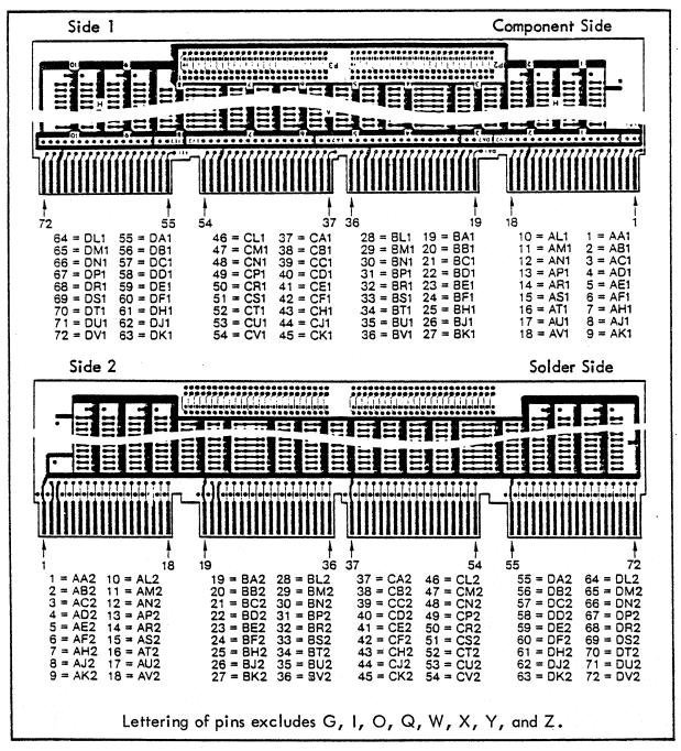
Figure 2-3 DEC-Compatible Module Pin Assignments
