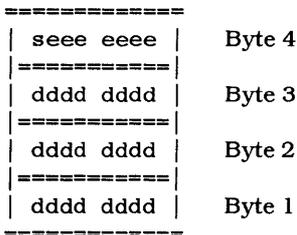
A BCD **double** has a sign bit, 11 bits of exponent, and 13 four-bit digits, as follows:
