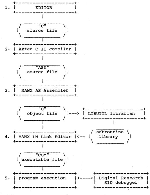
Figure 1. Developing "C" Programs with Aztec C II
