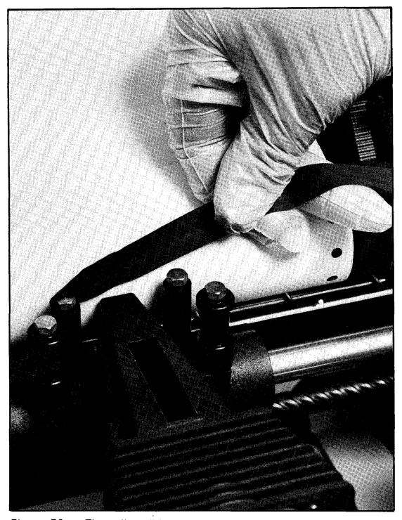
Figure 56. Threading ribbon around printer head
