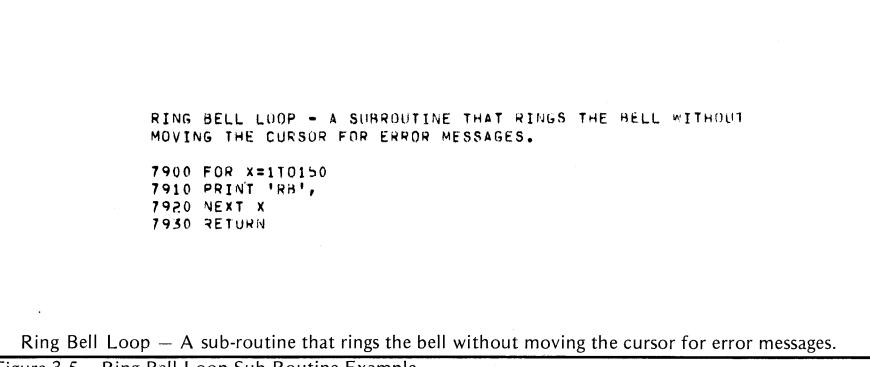
Figure 3-5. Ring Bell Loop Sub-Routine Example
