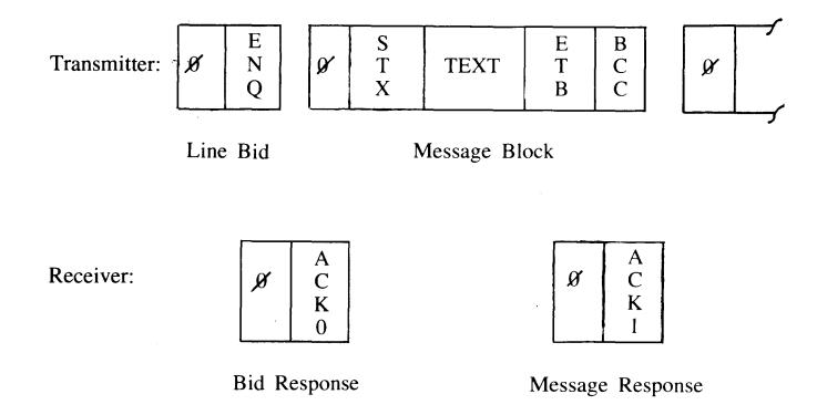
Figure 4. Line Bid Processing (Point-to-Point Operation)
