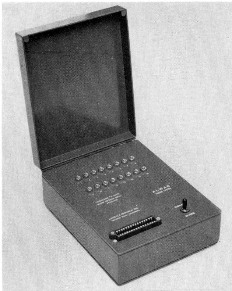
This tester is used for both input circuits and diode boards. Not only does it give a complete test of the diodes, but by means of one of the sixteen lights, an indication of the exact diode which is defective is indicated.
