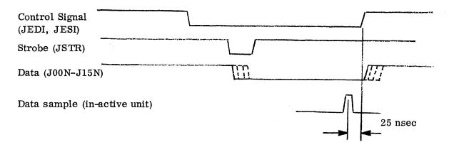
The selected device controller should enable the gating of data or status to the bus at the leading edge of Strobe JSTR, and disable it at the trailing edge of the control signal JEDI or JESI.
