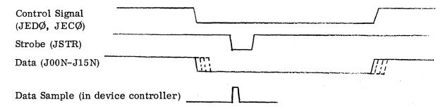
Any necessary delay in the data sample should be reflected in the acknowledge response JACK.
