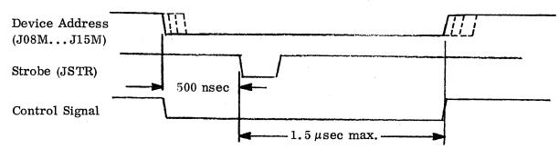
After the leading edge of Strobe, the Device Address lines will remain static as long as one of the four (4) control lines is active (1.5  $\mu$ sec max).
