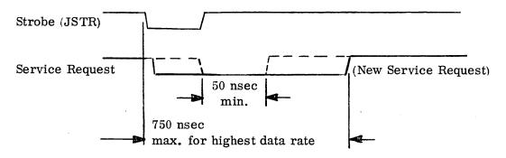
\* The "selected" strobe is determined by device controller address at the time a control signal is active.
