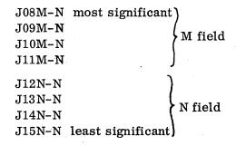
Device address is gated to the PDC in conjunction with the four (4) control signals, JEDI, JEDØ, JECØ, JESI, providing a unique address for each device controller. Each device controller must decode the address and respond no sooner than the leading edge of Strobe if it is to be selected. Typically 500 nsec is allowed for differential delays due to propagation and decode before Strobe occurs.
