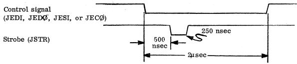
The width of the strobe will be 250 nsec. (Note: In this, and in all following discussions signal timing is specified with respect to the internal clock of the active unit, the CPU, MDC, or other. Delays due to logic and propagation will vary according to system configuration, and must not exceed the minimum time requirements where specified).
