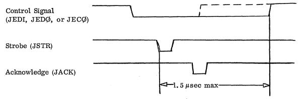
To achieve the highest data rate possible over the PDC, the active unit may use the JACK response to disable the control signal (and likewise disable device address and data); therefore, the device controller should not assume validity of data or address after the trailing edge of the control signal.
