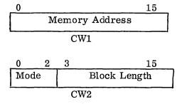
CW1 is incremented upon each word transferred and the block length is decremented each service request. Eight modes of operation are specified in the mode field, combinations of input or output, normal or burst, and word or byte.
