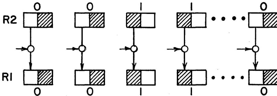
**Step 2. Flip-flops of R2 containing "1" cause corresponding flip-flops of R1 to set to "1" when voltage pulse is applied to gate tubes.**
