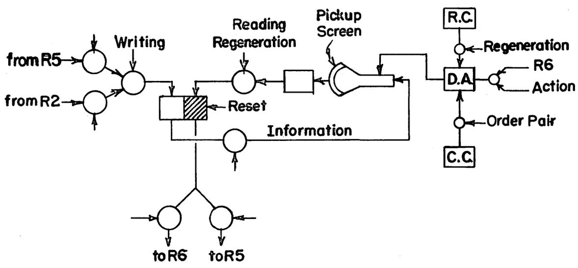
Fig. 5 Memory System. Abbreviations: D.A. deflection adder
