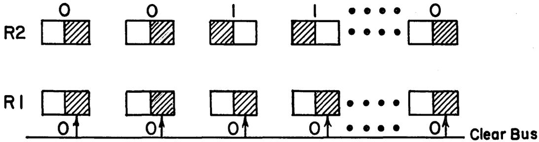
**Step 1. Clear R1 to ZEROS by voltage pulse on Clear Bus.**
