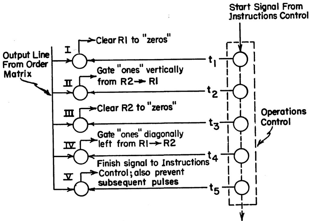
Fig. 9 Gate connections for a simplified order.
