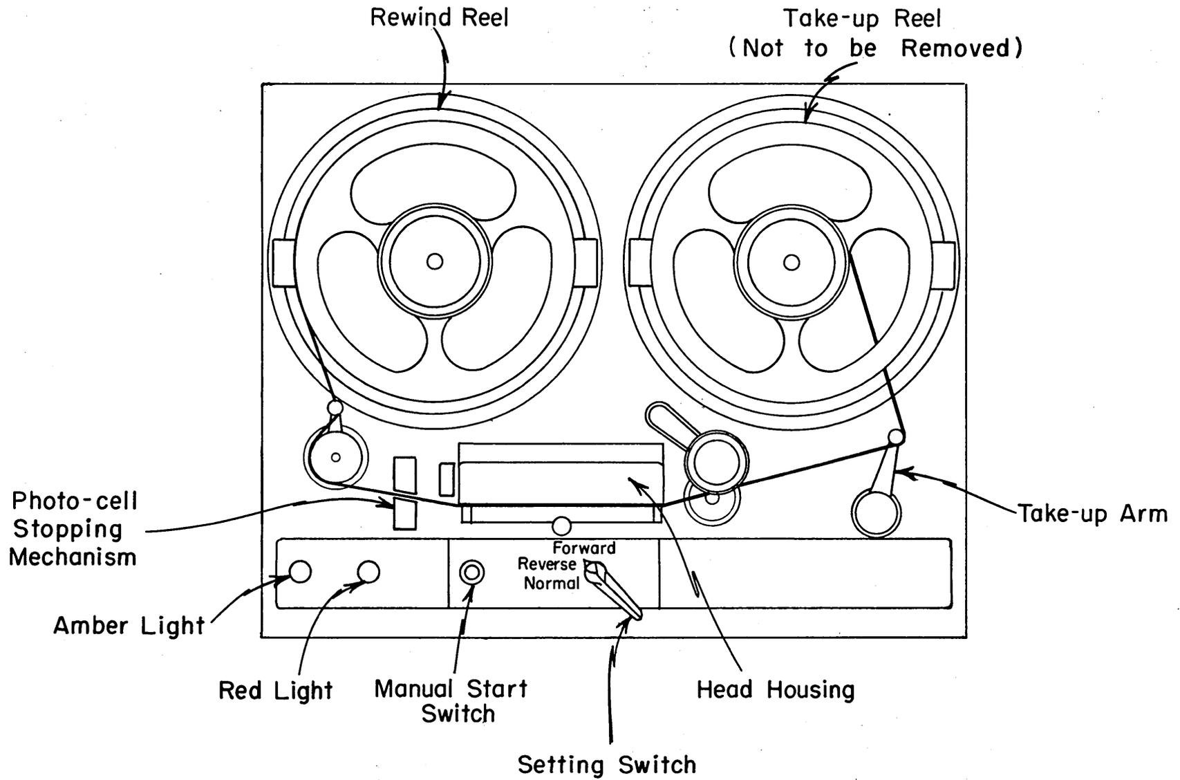
6. Wind several turns around the take-up reel. Wind the take-up reel until the take-up arm is in the position shown.
