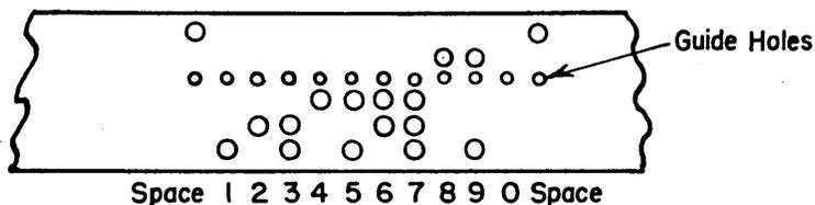
The punched holes correspond to the bit 1 and unpunched positions to 0. A sequence of such tetrads of binary digits is obviously not
