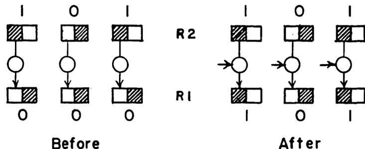
R1 has been previously cleared to 0's. The information in R2 is 101. When an appropriate voltage change is applied to the gate tubes, the first flip-flop of R1 will change its state to represent a 1, the second remains unchanged, and the third behaves like the first. R1 will then have received the information 101.
