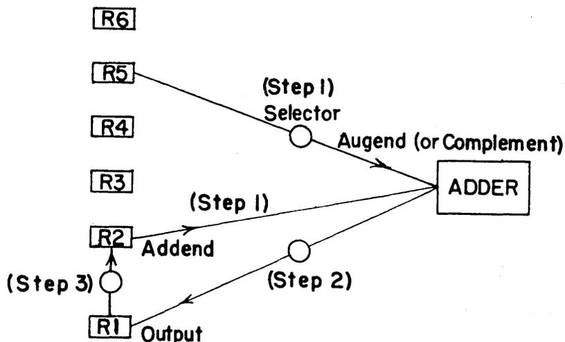
To recapitulate, the addition process (or subtraction) involves adding to the number in R2 the number (or its complement) in R5. The sum appears finally in R2. The fact that the sum replaces one of the terms is very convenient for the multiplication and division processes, where the sum is the partial product or the partial remainder, respectively. The multiplicand or the divisor resides accordingly in R5.
