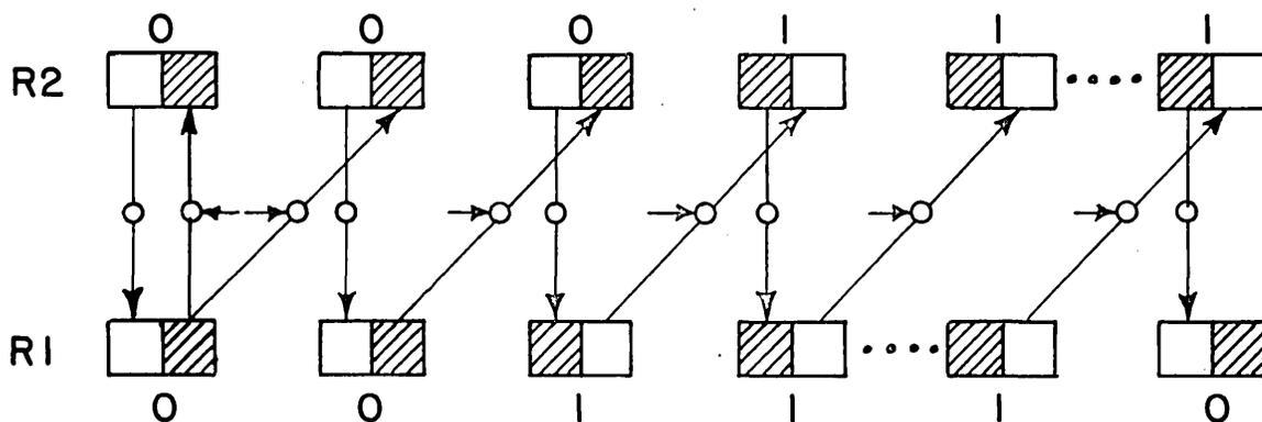
Step 4. Flip-flops of R1 containing "0" cause corresponding flip-flops of R2 to set to "0".
