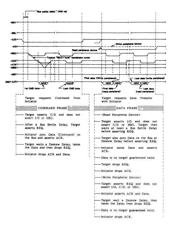
Figure 1-4. SCSI Timing Diagram, Command, and Data Phases
