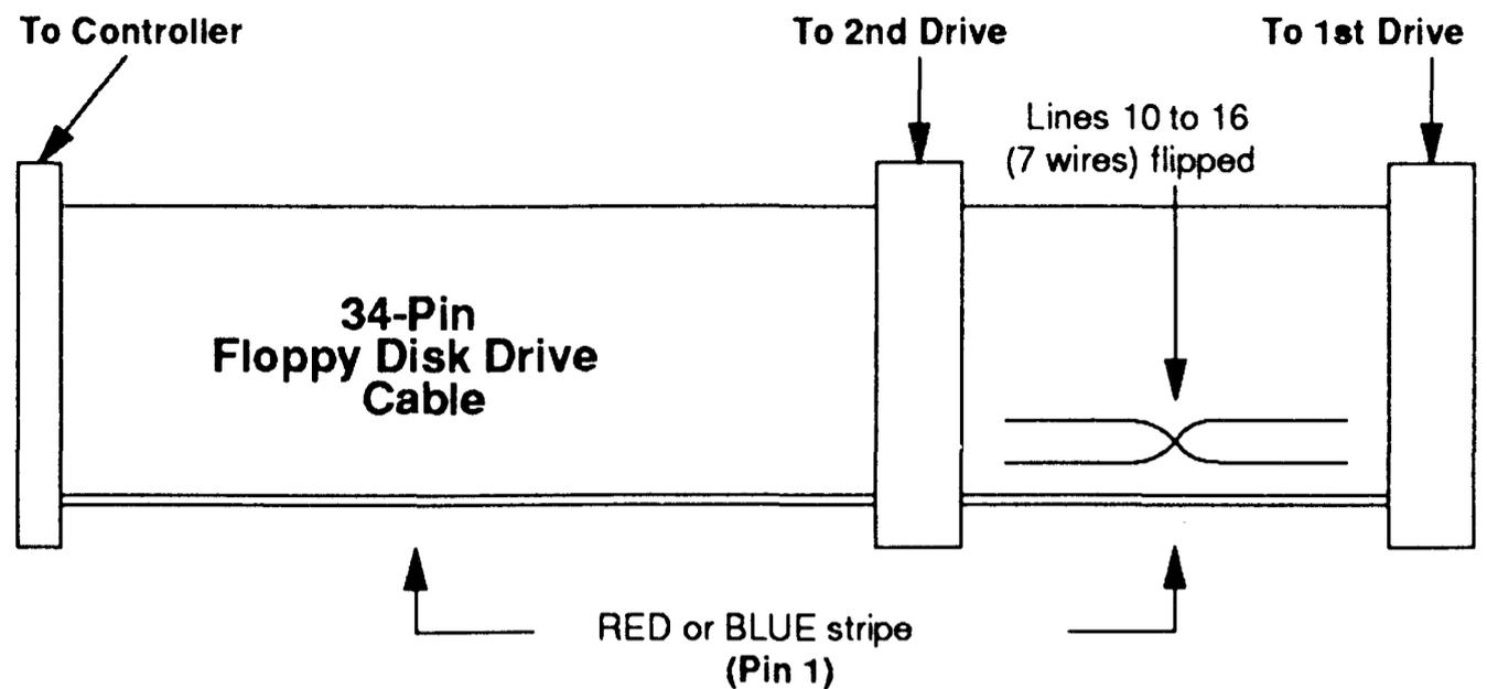
Attach the end of the cable to the first floppy disk drive (drive A:). Make sure the it attaches to the connector on the end of the cable and that the red or blue stripe on the cable faces the correct direction.
