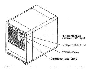
Figure 2-5. Lowboy Electronics Cabinet Main Components
