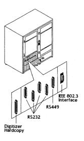
Figure 2-8. Two-Bay Electronics Cabinets Ports
