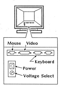
Figure 1-3. 27-Inch Monitor Ports
