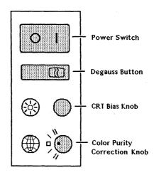
Figure 1-4. 27-Inch Monitor Control Panel
