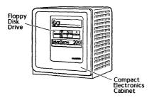
Figure 2-1. Cube Electronics Cabinet Main Components
