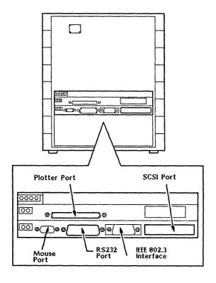
Figure 2-2. Cube Electronics Cabinet Ports
