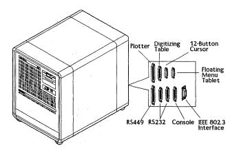
Figure 2-6. Lowboy Electronics Cabinet Ports
