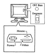
Figure 1-2. 15/19-Inch Monitor Ports
