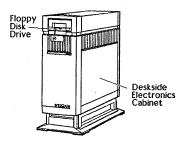
Figure 2-3. Suitcase Electronics Cabinet Main Components
