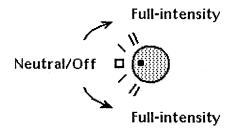
Figure 1-5. Color Purity Correction Knob Settings
