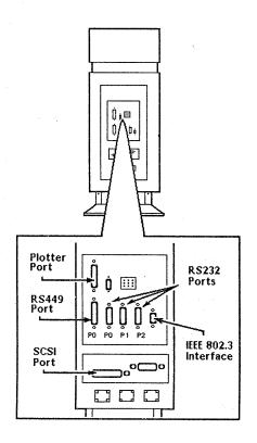
Figure 2-4. Suitcase Electronics Cabinet Ports
