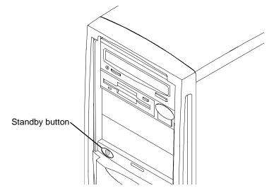
The power button is a momentary contact switch, changing system states every time the button is pressed.
