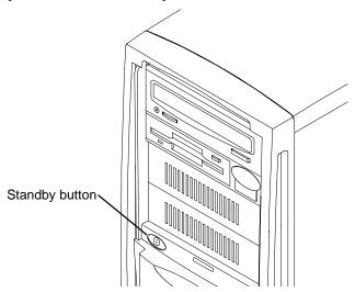
The power button is a momentary contact switch, changing system states each time the button is pressed.
