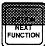
Advances the LCD to the next available second function option. The selected function and its current value will be displayed in the LCD.
