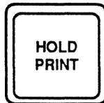
Interrupts printing and **activates all keys**. If the printer is in OPTION mode, pressing this key will cause the printer to return to HOLD without altering the indicated function. It will also return you to the beginning of the second function option menu.
