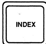
Inserts one blank line. If the position goes beyond the bottom of the page as defined by the forms length parameter, one page will be fed in the printer.\*
