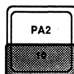
These keys are referred to as Program Attention Keys. If the SCS (SNA Character String) feature is operational on your Laser 8 unit, these Program Attention keys can be selected while in SCS mode to transfer printing control to the application program.
