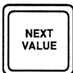
Displays the next value choice available for a specific function. The **NEXT VALUE** key should be used with the following functions: Case, Spacing, LPI, CPI, Page Size, Orientation, and Hopper .
