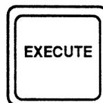
Tells the printer to perform the selected function and returns the printer to **HOLD**. If a new value for a parameter has been set, that value takes effect when **EXECUTE** is pressed. The new value will not remain in the printer's memory after the printer is powered off.
