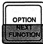
Enters the printer into second function mode activating all second functions and second function options. Read the following section for specific instructions on using this key.
