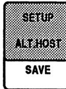
Allows you to change factory set defaults. Pressing this key permanently saves the currently selected option value as the new default. This new setting, called a user default, will be used at the next power on. The printer will perform a power on reset following a SAVE. See page 65 for details.
