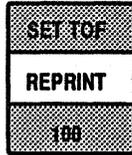
Causes the printer to reprint the contents of the print buffer.
