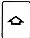
In menu mode the UP ARROW is used to scroll forward through the individual option values. See page 55 for the Primary mode function of this key.
