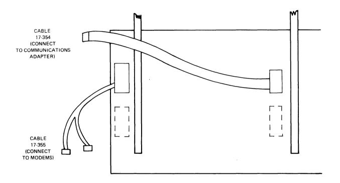
Figure 2A. Cable Connections (02-380A20)
