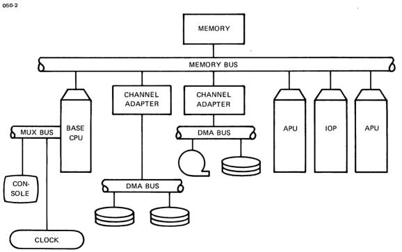
Figure 1-2 Configuration of a Typical Multiprocessing System
