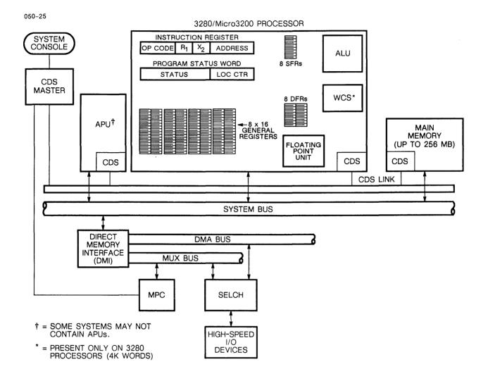
Figure 1-3 Configuration of a Typical 3280/Micro3200 System
