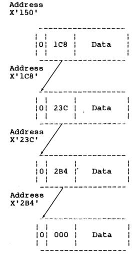
Figure 6-10 Multiple Buffer Chain
