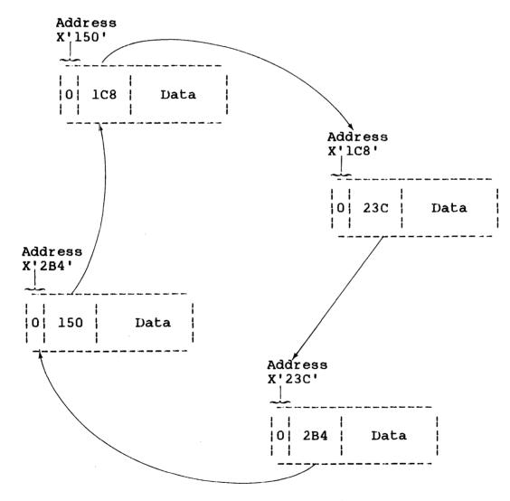
Figure 6-9 Multiple Buffer Ring
