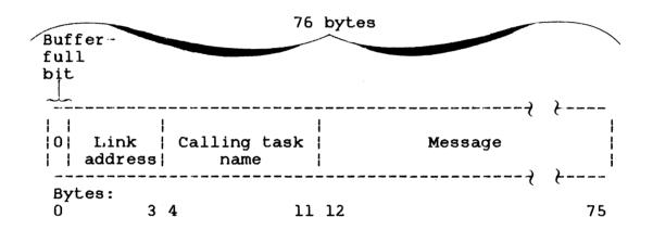
Figure 6-6 Message Buffer Format for Directed Task
