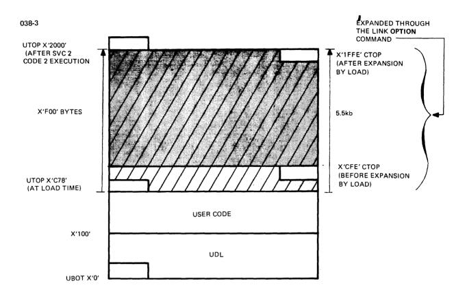
Figure 3-7 Task Impure Segment for SVC2 Code 3
