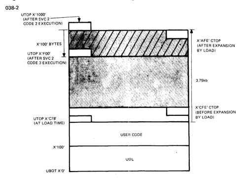
Figure 3-5 Task Impure Segment for SVC2 Code 2, Option X'80'
