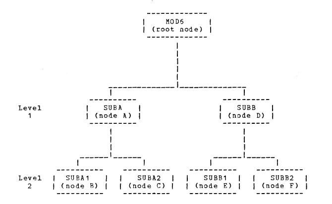
Figure 4-1 Sample Overlay Structure
