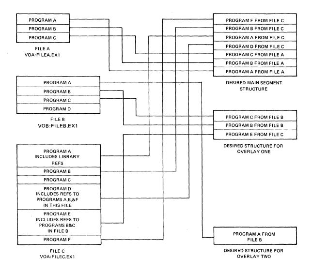
Figure D-2 Graphic Description of a Task with Two Overlays
