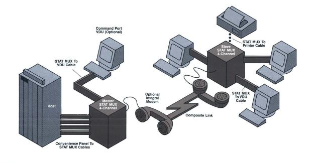
Product Description The Perkin-Elmer Point-to-Point (Pt-Pt) Statistical Multiplexor (STAT MUX) is a high-speed data concentrator offered with optional integral modem. The Pt-Pt STAT MUX provides a communications link with up to 16 channels between a remote site and a central host.
