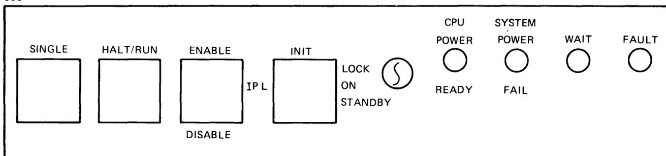
Figure 2-1 System Control Panel
