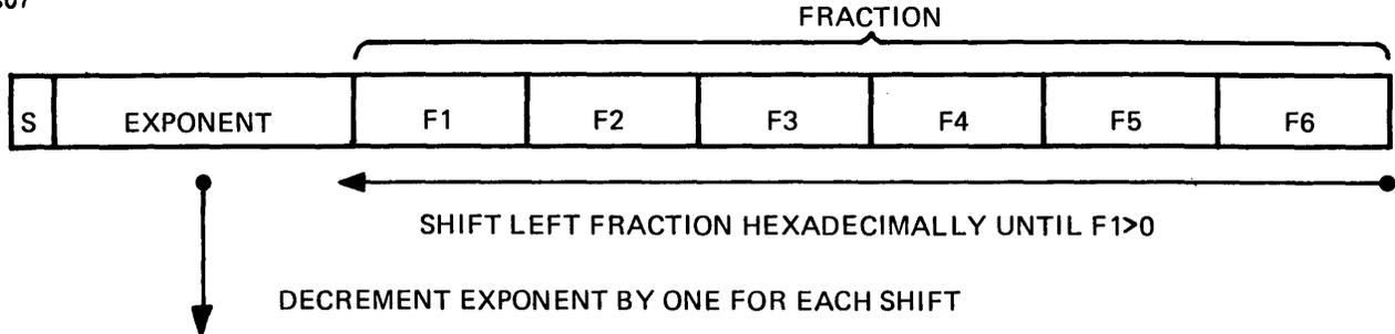
Except for the load instructions, all floating-point operations assume and require normalized operands for consistent results. The load instructions normalize an unnormalized operand.
