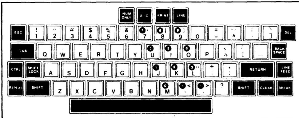
Figure 2-2 Model 550 Keyboard Layout
