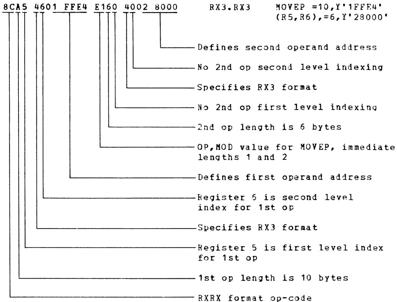
In this example, both members of the RXX instruction use the RX3 format. Double indexing is specified for the first member and no indexing is specified for the second member. The first operand address is X'1FFE4' plus the contents of index registers 6 and 5. The second operand address is X'28000'. The length of each of the first operand is ten bytes and the second operand is six bytes.
