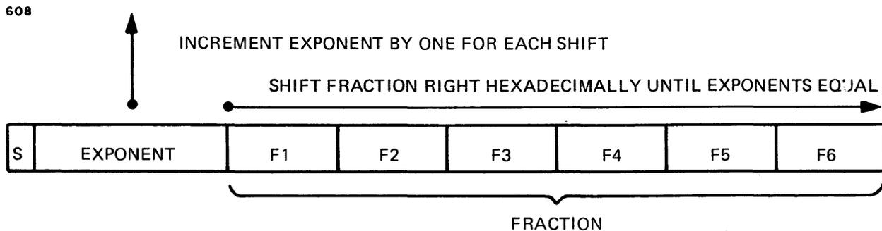
During floating-point addition and subtraction, the two floating-point operands are equalized.
