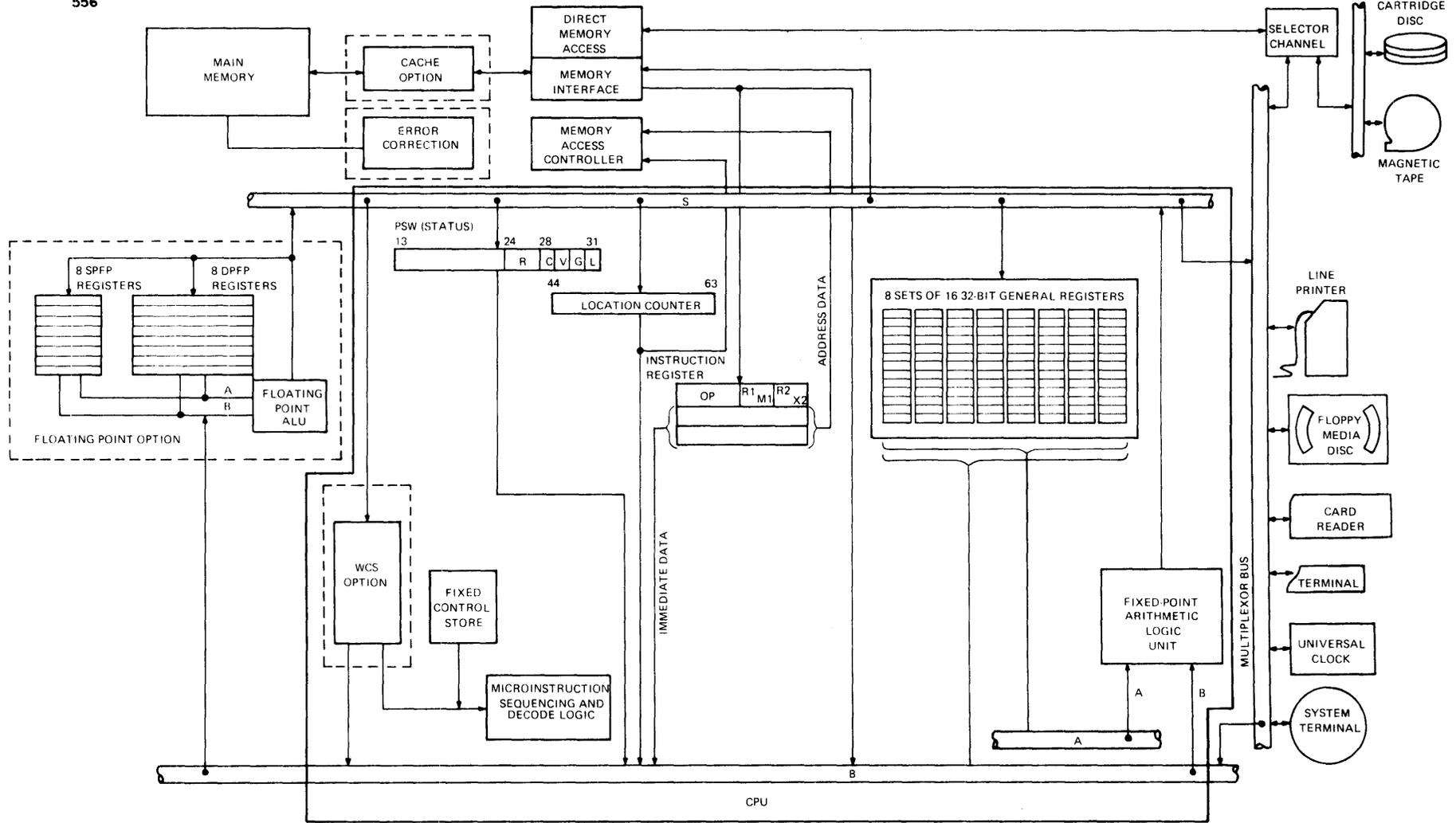
Figure 1-1 Model 3220 Processor Block Diagram
