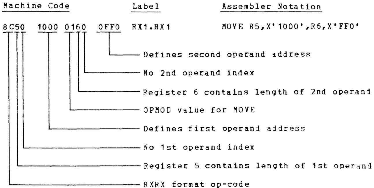
In this example both members of the RXXR instruction use the RX1 format. No indexing is specified for either member so the first operand address is X'1000', and the second operand address is X'0FF0'.
