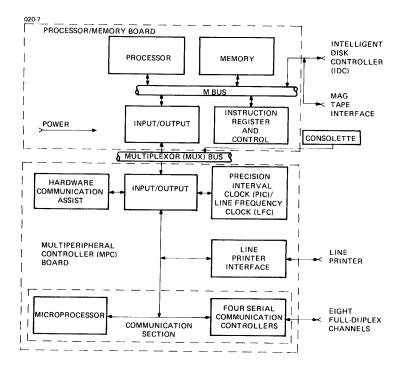
Figure 2-1 Model 3205 System Boards
