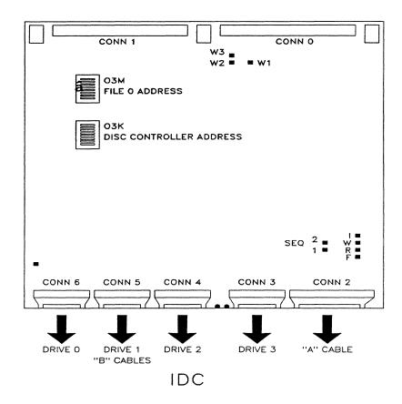
CONTROLLER ADDRESS. Open=1, Closed=0. Example: All open except switch 6 - x'FB.
