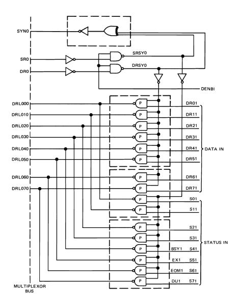
Figure 5-17. Data and Status Input, Logic Diagram
