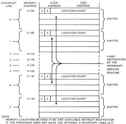
THE FIRST INSTRUCTION OF THE NEW PROGRAM CORRESPONDING TO INTERRUPT LINE 0 WOULD BE AT LOCATION X'102'
