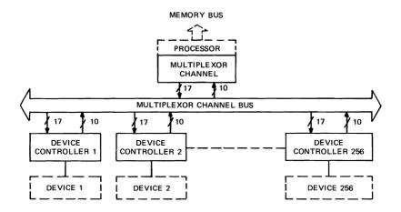
Figure 5-2. Multiplexor Channel, Block Diagram
