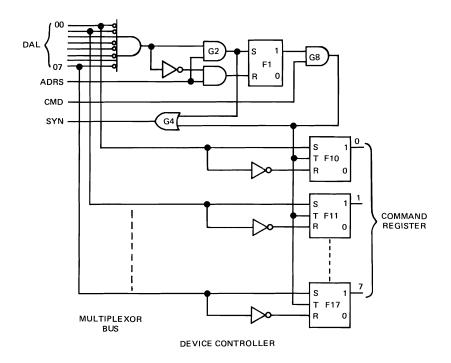
Figure 5-7. Device Controller Logic for the Output Command Instruction
