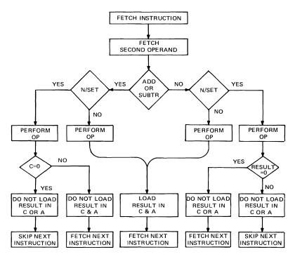
Figure 4-10. Arithmetic and Logical Memory Reference Instructions Flow Chart
