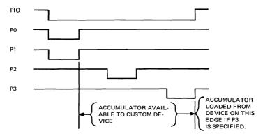
Figure 4-7. Pulsed I/O Timing
