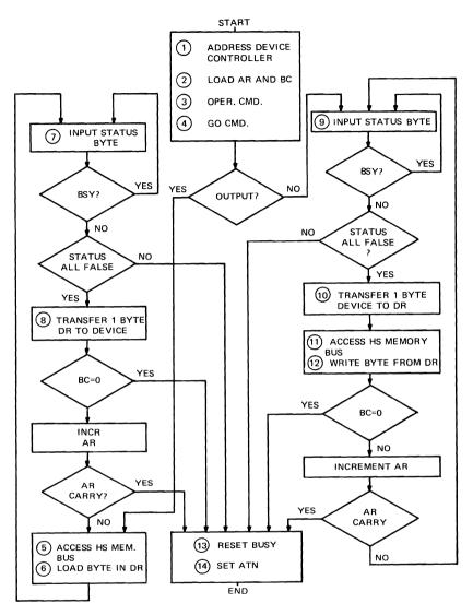
Figure 5-4. Selector Channel, Flow Chart
