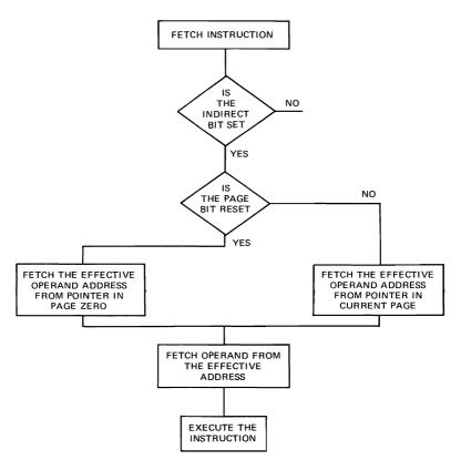
Figure 3-4. Flow Chart - Indirect Addressing Mode
