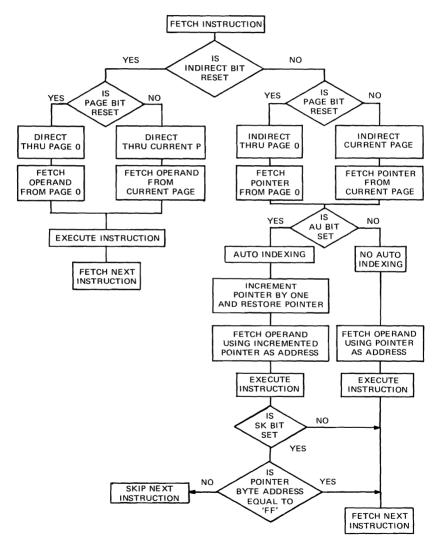
Figure 3-6. Flow Chart - Addressing Modes/Auto Indexing
