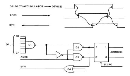
Figure 5-6. Device Controller Logic For The Address Instruction
