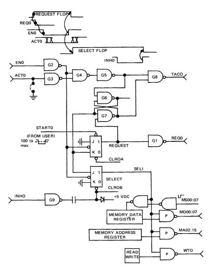
Figure 6-7 Daisy-Chain Select Request Circuits
