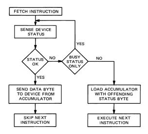
Figure 4-5. Write Data and Skip Flow Chart
