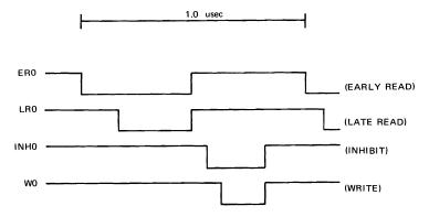
The Write (WTO) Line defines whether the current memory cycle is a Read or a Write cycle.
