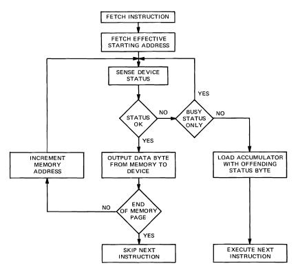
Figure 4-6. Write Block Flow Chart
