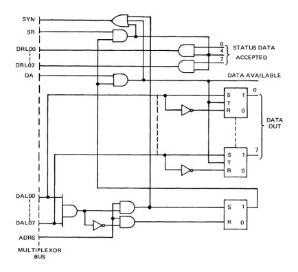
Figure 13. Device Controller Logic (Write Data and Skip and Write Block Instruction)
