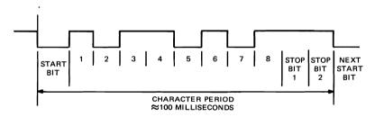
The Start Bit corresponds to a binary one. The Stop Bits correspond to binary zeros. The data bits correspond to eight level ACSII code. The Start Bit and the two Stop Bits have no significant data content. They are used only to identify the beginning and the end of a character period.
