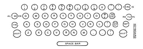
Figure 11-3. ASR 33 Teletype Keyboard Layout
