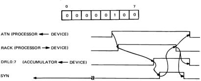
This instruction is used to identify which of up to 256 device controllers interrupted the Processor over the common Attention (ATN) Line.
