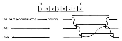
Figure 5-8 provides the device controller logic for the Write Data Instruction.
