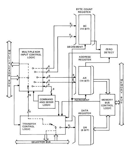
Figure 5-3. Selector Channel, Block Diagram
