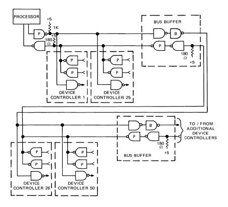
Figure 5-15. Multiplexor Channel Bus Buffers
