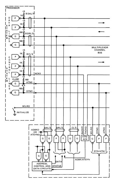
Figure 5-14. I/O Bus Communication Circuits, Logic Diagram
