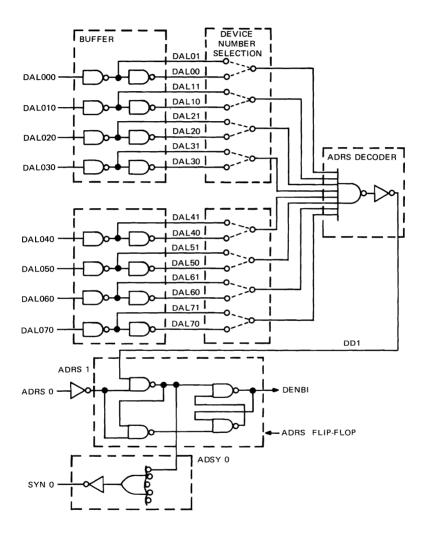
Figure 5-16. Device Addressing, Logic Diagram
