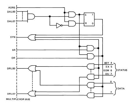
Figure 5-12. Device Controller Logic (Read Data Skip or Read Block Instruction)
