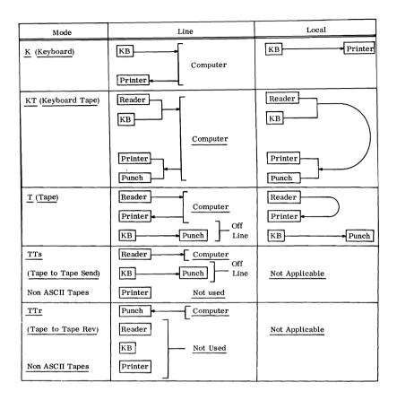
In the STOP position, tape motion can be controlled by program, assuming the teletype power switch is in the LINE position. The specific control characters which affect the reader are X-ON (X'91') which starts the tape motion, and X-OFF (X'93') which stops tape motion.
