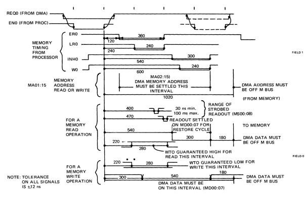
Figure 6-6. Model 1 Memory Bus Timing
