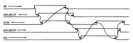
The WDS instruction is a combined Sense Status and Write Data instruction where the Processor tests the device status and, when the device is ready, sends a data byte to the device. See Figure 5-13.
