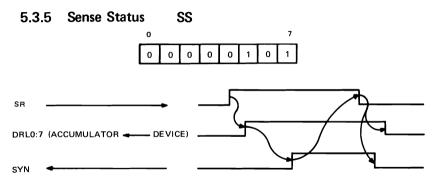
The Sense Status instruction transfers an eight bit Status Byte from the addressed device controller to the Processor. Status bits take on different meanings for different device controllers. In general, however, data may only be transferred between the Processor and the device when the status of that device is all zeros. Figure 5-9 provides the Device Controller Logic for the Sense Status Instruction.
