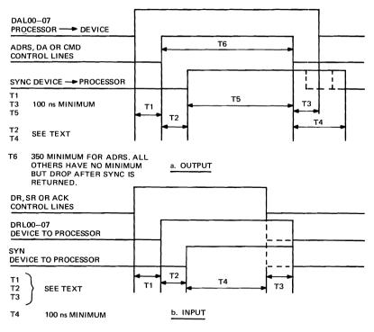
Figure 5-21. Multiplexor Channel Timing
