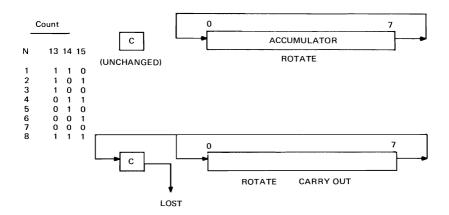
Figure 4-4. Example of Rotate Instruction
