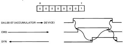
Figure 5-7 provides the device controller logic for the output Command Instruction.
