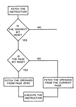
Figure 3-3. Flow Chart - Direct Addressing Mode
