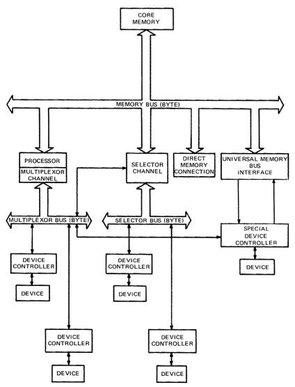
Figure 5-1. Systems Interface, Block Diagram
