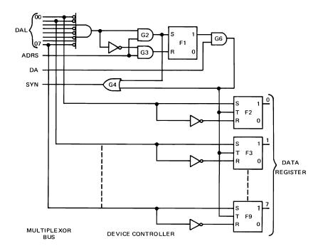
Figure 5-8. Device Controller Logic for the Write Data Instruction
