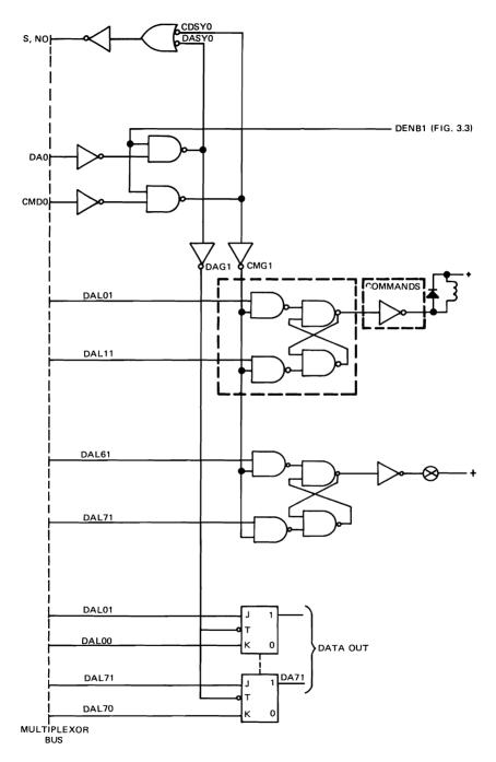
Figure 5-18. Data and Command Output, Logic Diagram
