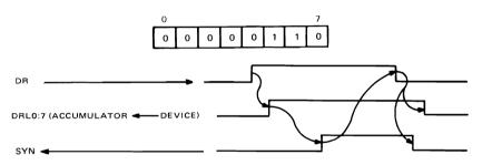
Figure 5-10 provides the device controller logic for the Read Data Instruction.
