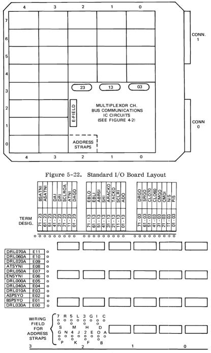
Figure 5-23. Standard I/O Board Field Layout
