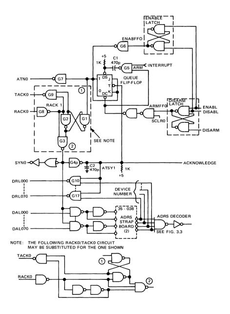
Figure 5-19. Interrupt Control, Logic Diagram
