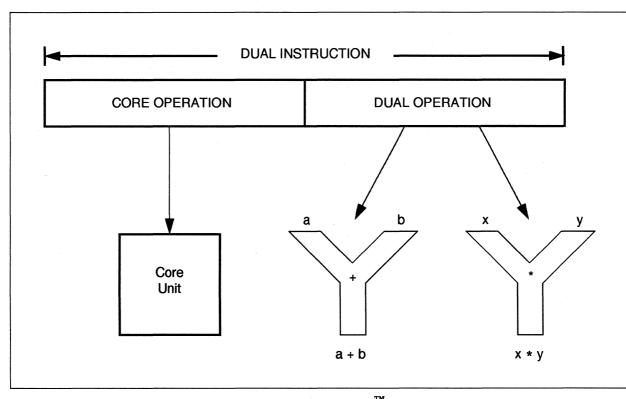
Figure B-2. Parallel Activities of i860<sup>™</sup> Microprocessor
