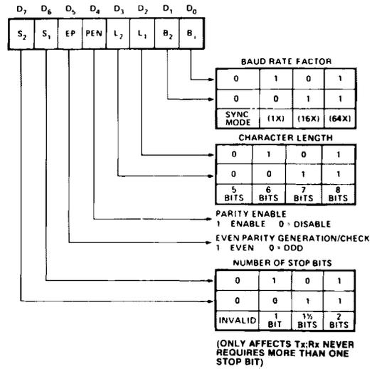
Figure 3-3. USART Asynchronous Mode Instruction Word Format
