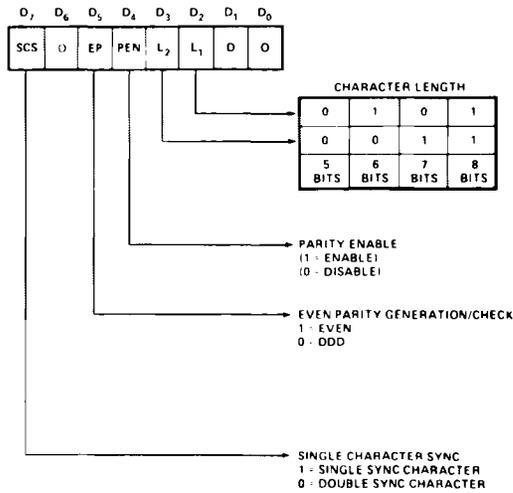
Figure 3-1. USART Synchronous Mode Instruction Word Format
