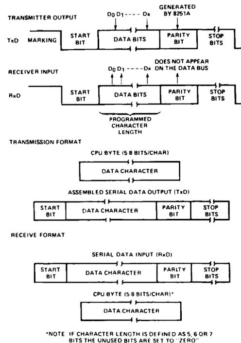
Figure 3-4. USART Asynchronous Mode Transmission Format
