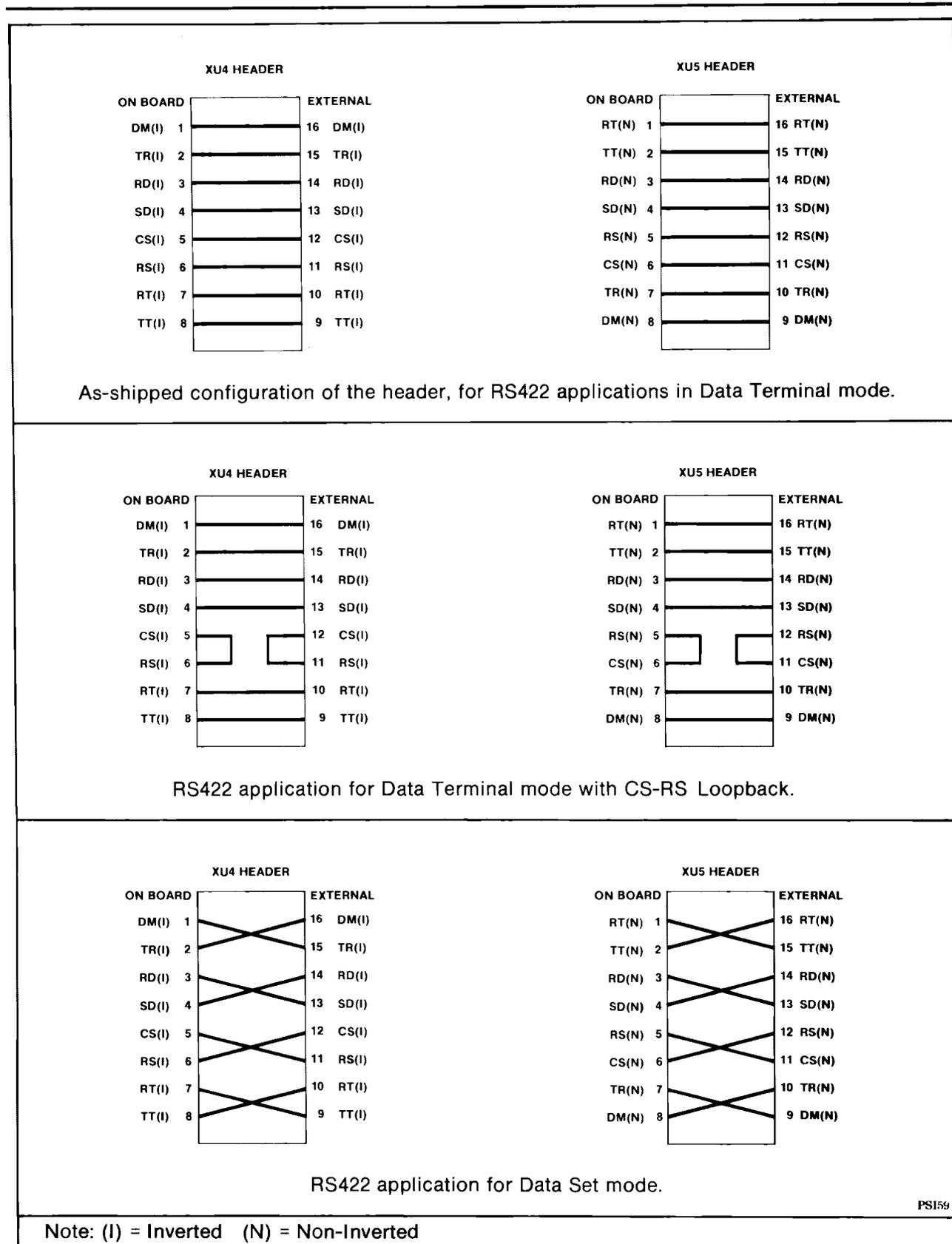
Figure 2-4. Header Wiring For RS422
