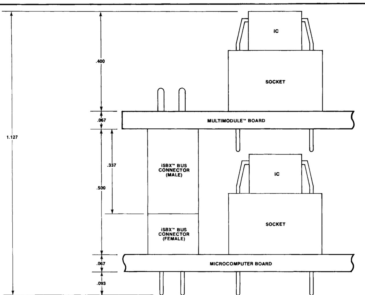
Figure 2-2. Mounting Clearances (Inches)
