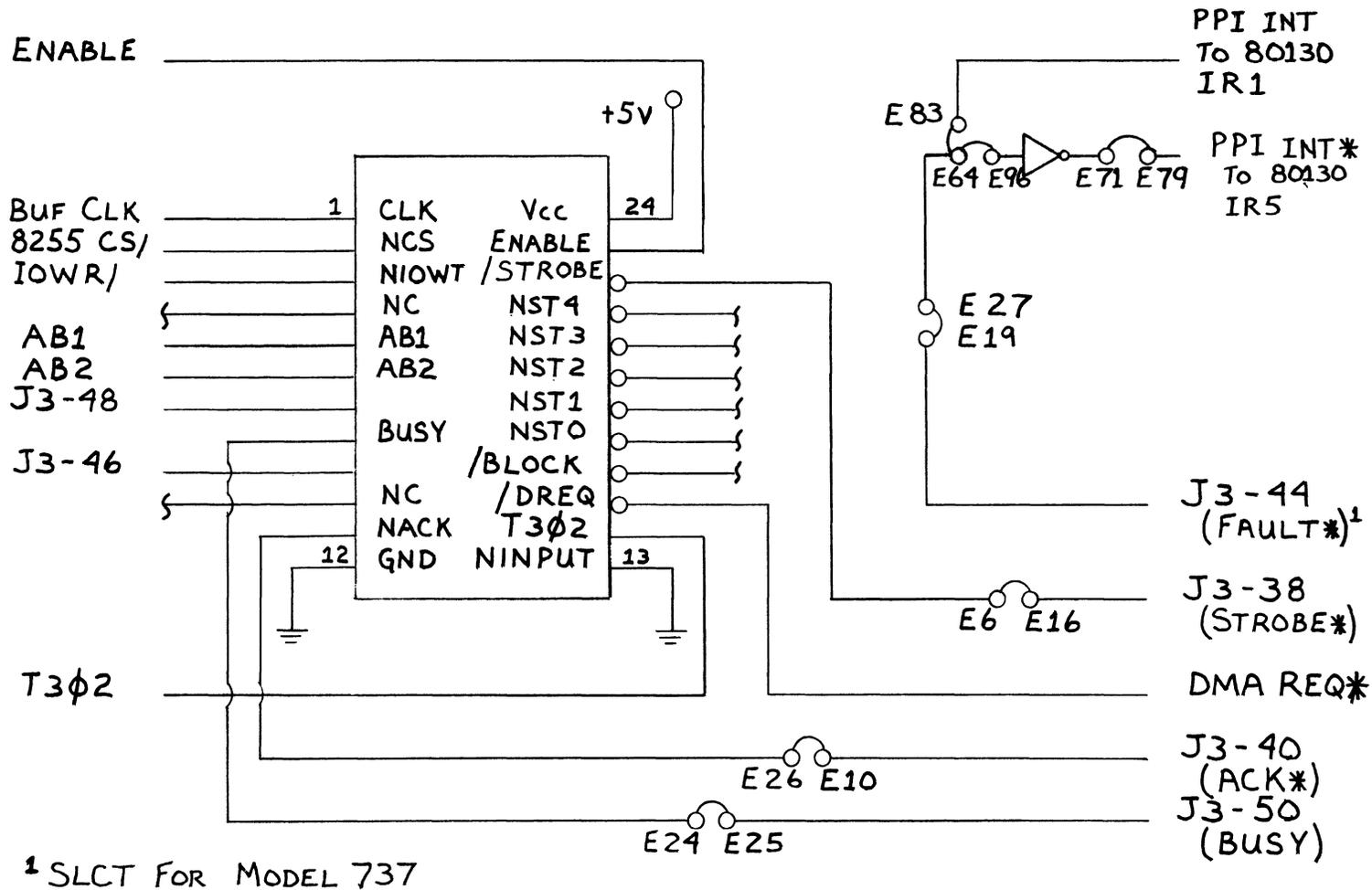
Figure C-10. Centronics PAL with Jumper Connections
