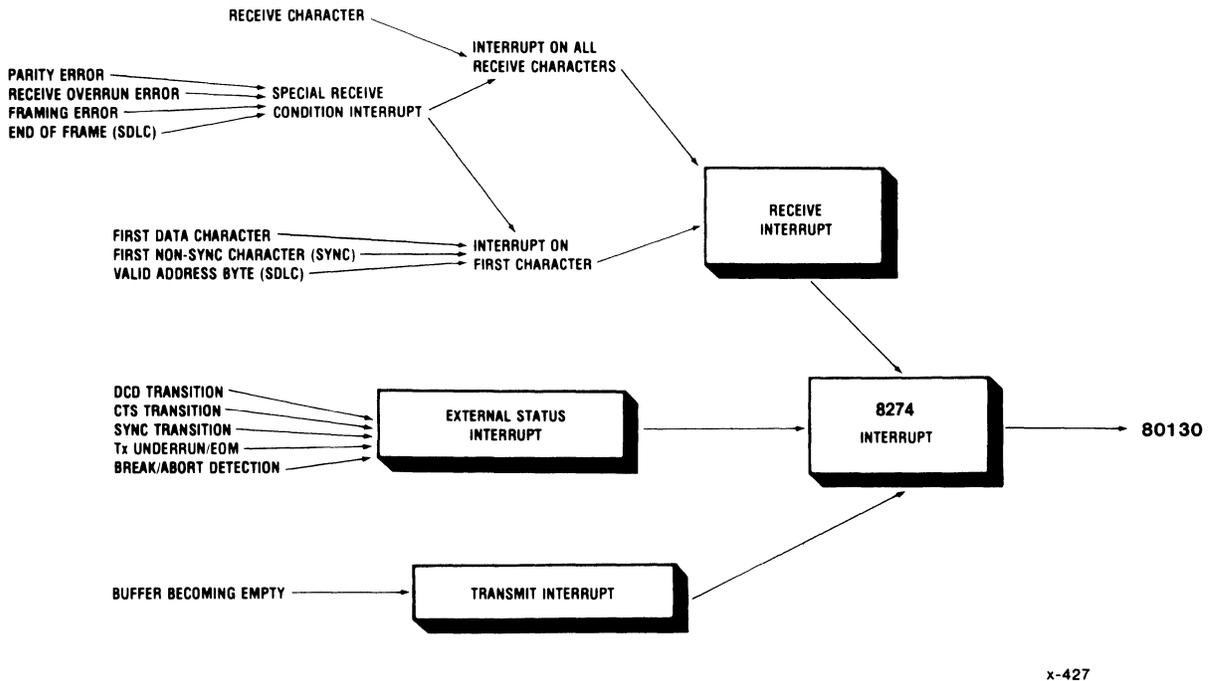
Figure 4-6. Interrupt Structure
