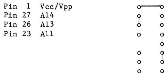
Figure D-4. Jumper Matrix Configurations for EPROM Devices (continued)
