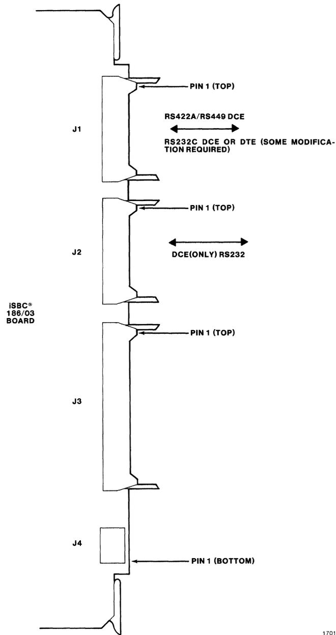
Figure 2-7. Physical Locations of Connectors and Pin 1 Assignments
