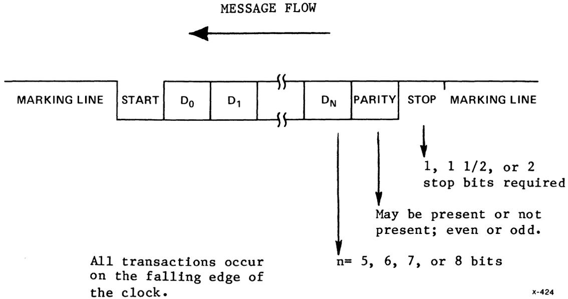
Figure 4-3. Asynchronous Message Format
