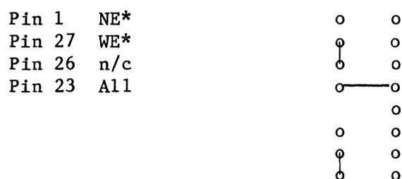
Figure D-6. Jumper Matrix Configurations for EEPROM Devices
