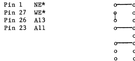
Figure D-5. Jumper Matrix Configurations for NVRAM Devices
