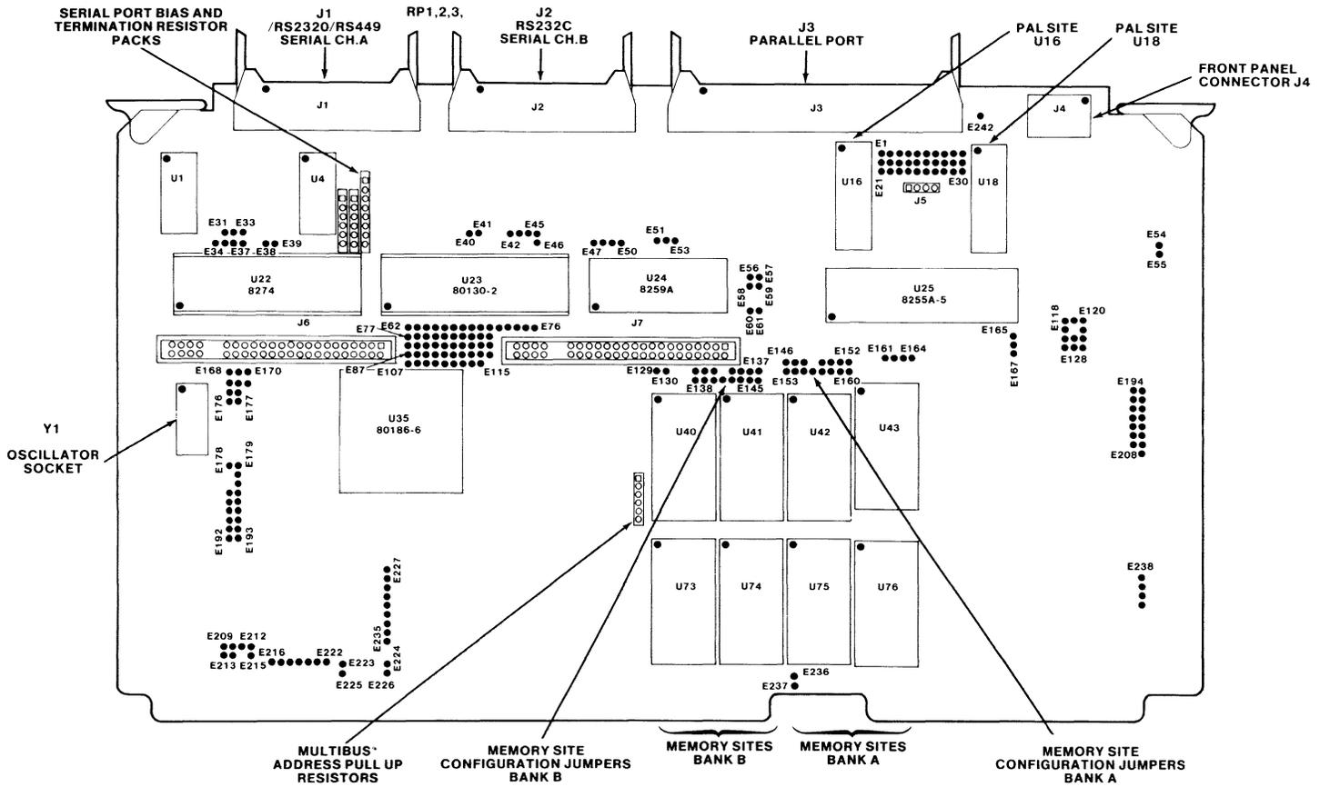
Figure 3-1. User-Furnished Components on the isBC® 186/03 Board
