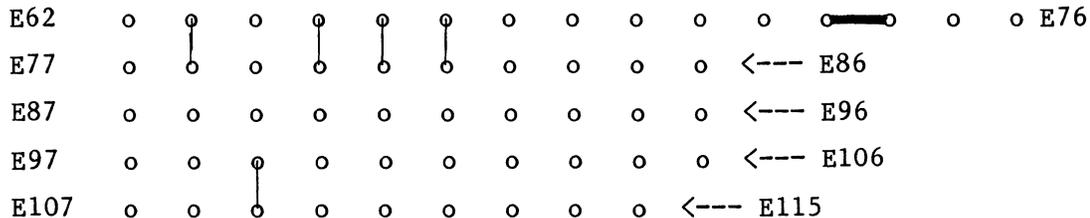
Figure 2-6. Default Configuration Of Interrupt Jumper Matrix
