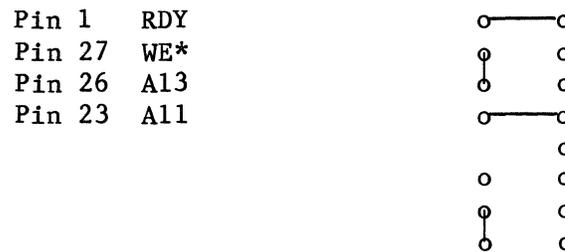
Figure D-3. Jumper Matrix Configurations for iRAM Devices
