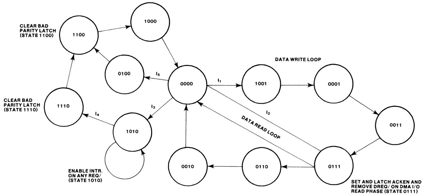
Figure C-4. SCSI State Machine Diagram
