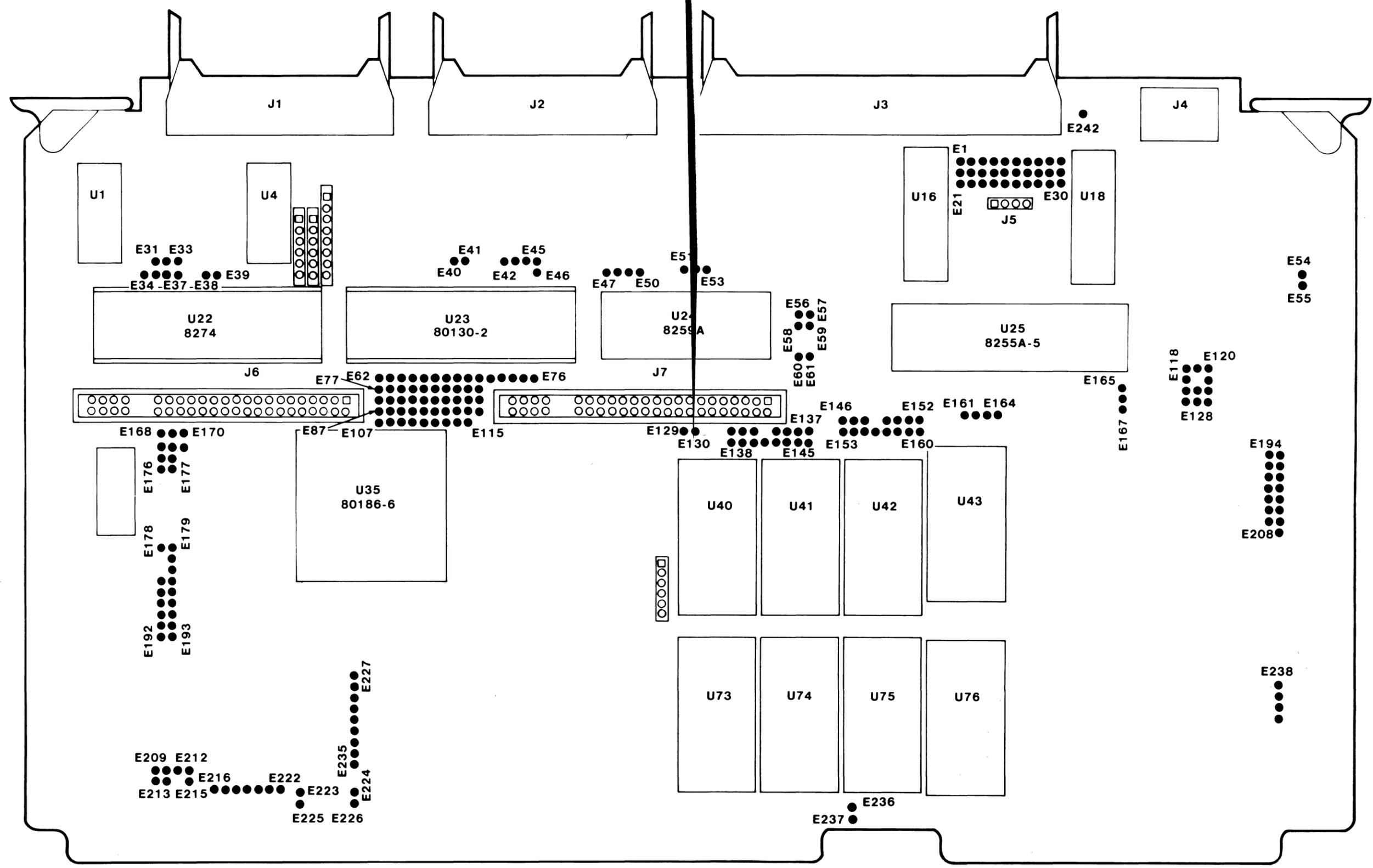
Figure A-1. Jumper Post Location Diagram
