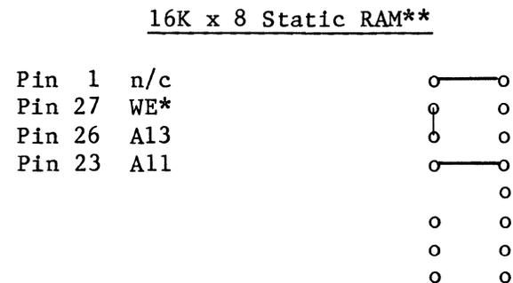
Figure D-2. Jumper Matrix Configurations for Static RAM Devices
