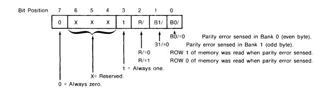
Figure 3-1. Parity Flag Register Format
