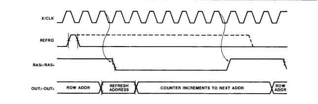
Figure 4-4. External REFRESH Command Timing
