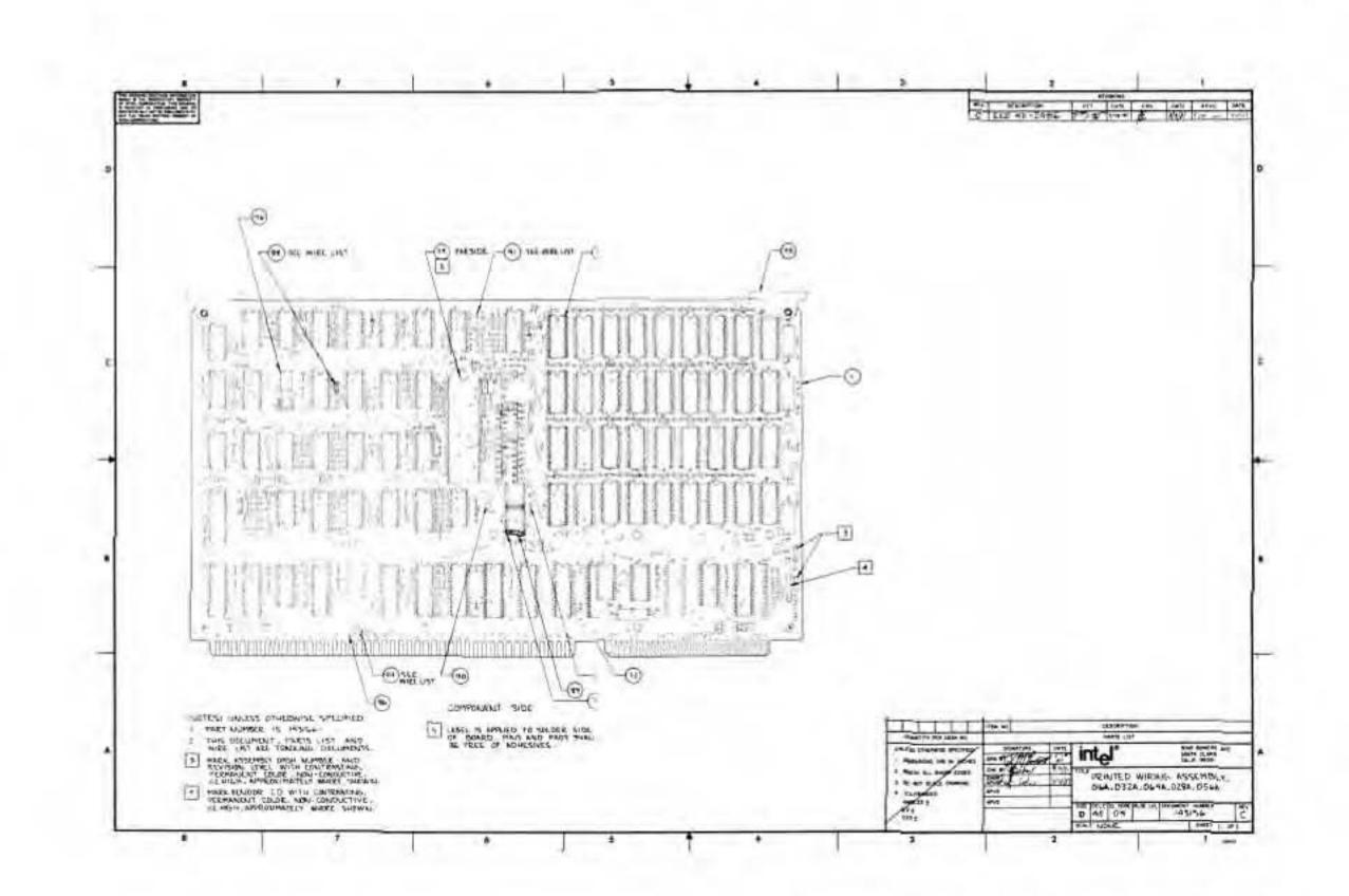
Figure 5-2. iSBC 016A/032A/064A/028A/056A<sup>TD</sup> RAM Boards Parts Location Diagram
