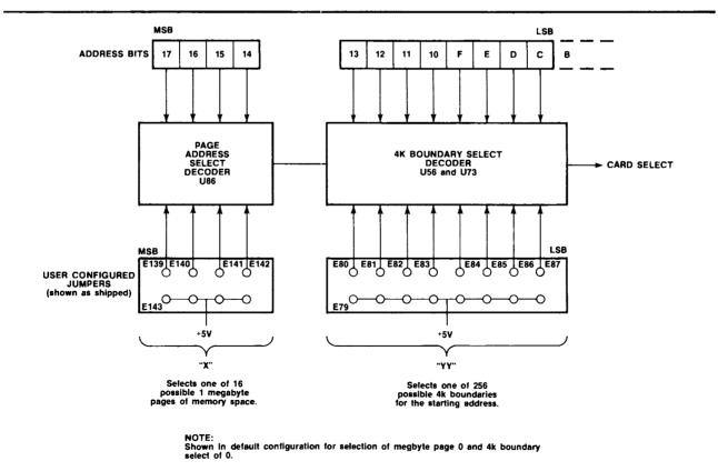
Figure 2-4. Address Selection Jumper Configuration
