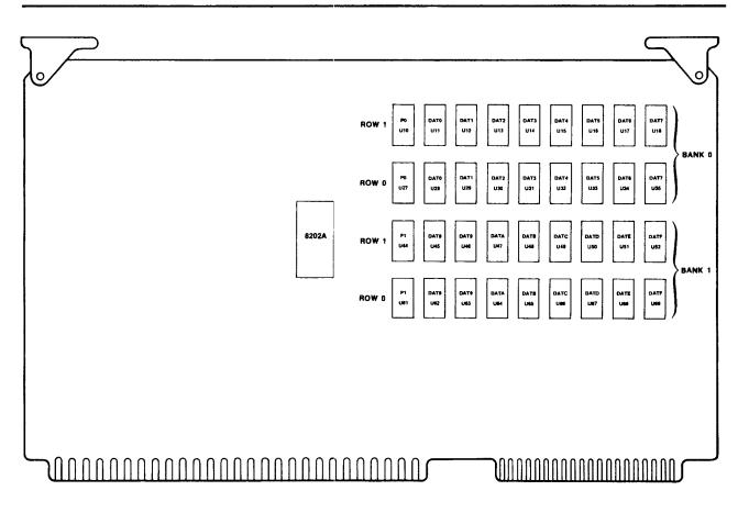
Figure 4-2. Memory Array Layout
