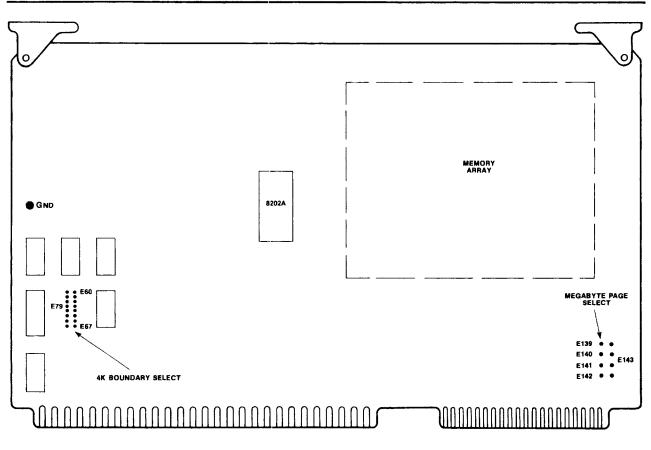
Figure 2-3. Memory Address Jumper Location Diagram
