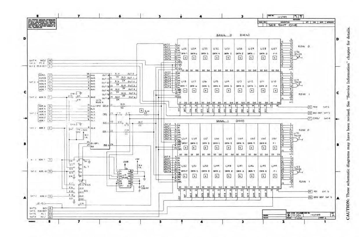
Figure 5-3. iSBC 016A/032A/064A/028A/056A™ RAM Boards Schematic Diagram (Sheet 3 of 5)
