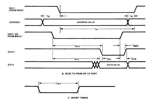
Figure 2-2. Multibus Timing For I/O READ and I/O WRITE operations
