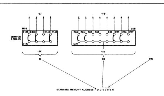
Figure 2-5. Address Jumper Configuration Example
