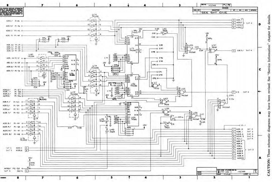
Figure 5-3. iSBC 016A/032A/064A/028A/056A<sup>™</sup> RAM Boards Schematic Diagram (Sheet 2 of 5)
