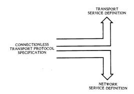
A document (ISO/TC 97/SC16N, February 1983) entitled "Working Draft for an addendum to the Transport Protocol Specification Covering Connectionless Data Transmission" Specifies transport architecture for connectionless systems. It is the specification followed by release 1 of the iNA960 and the source of this section.
