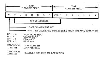
Figure 2-5(a). DSAP and SSAP Address Field Formats
