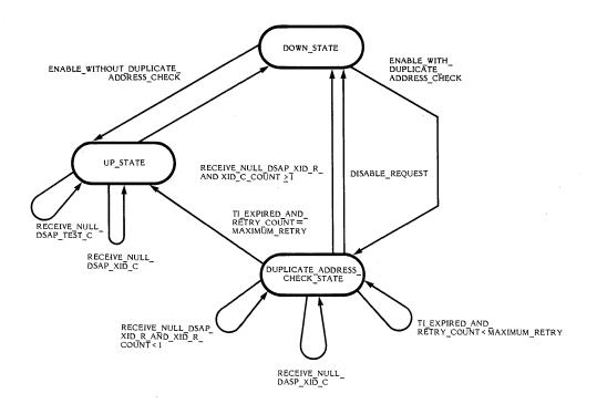
Figure 2-11. Station Component State Diagram
