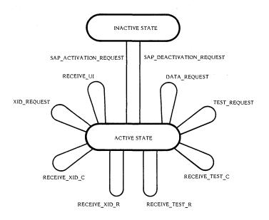
Figure 2-12. Link Service Access Point State Diagram
