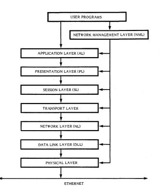
Figure 1-1. The Layered Network Architecture
