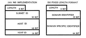
In Release 1 of iNA 960, the internet address consists of a 32-bit subnet identifier (ID), a 48-bit Ethernet host ID, and a 16-bit NSAP ID. The Ethernet ID and the NSAP ID form the domain specific identifier, which is an issue determined within the Ethernet community.
