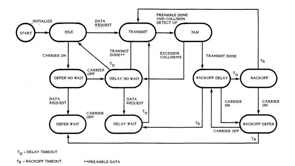
Figure 2-19. Transmit Component State Diagram
