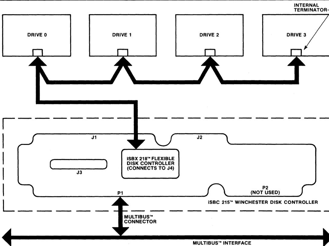
**Figure 1-2 Typical Multiple Drive System Using Flexible Disk Drives and iSBX 218™ Flexible Disk Controller**
