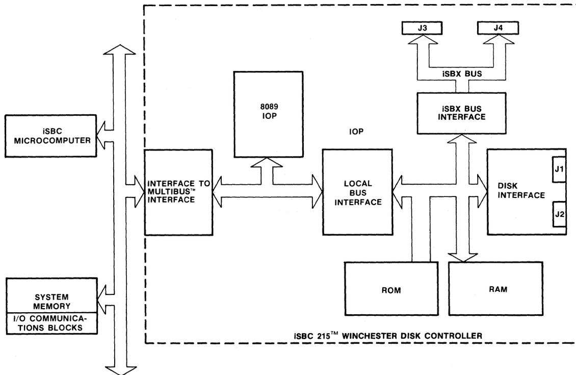
Figure 4-2. Simplified Block Diagram of iSBX 215™ Controller
