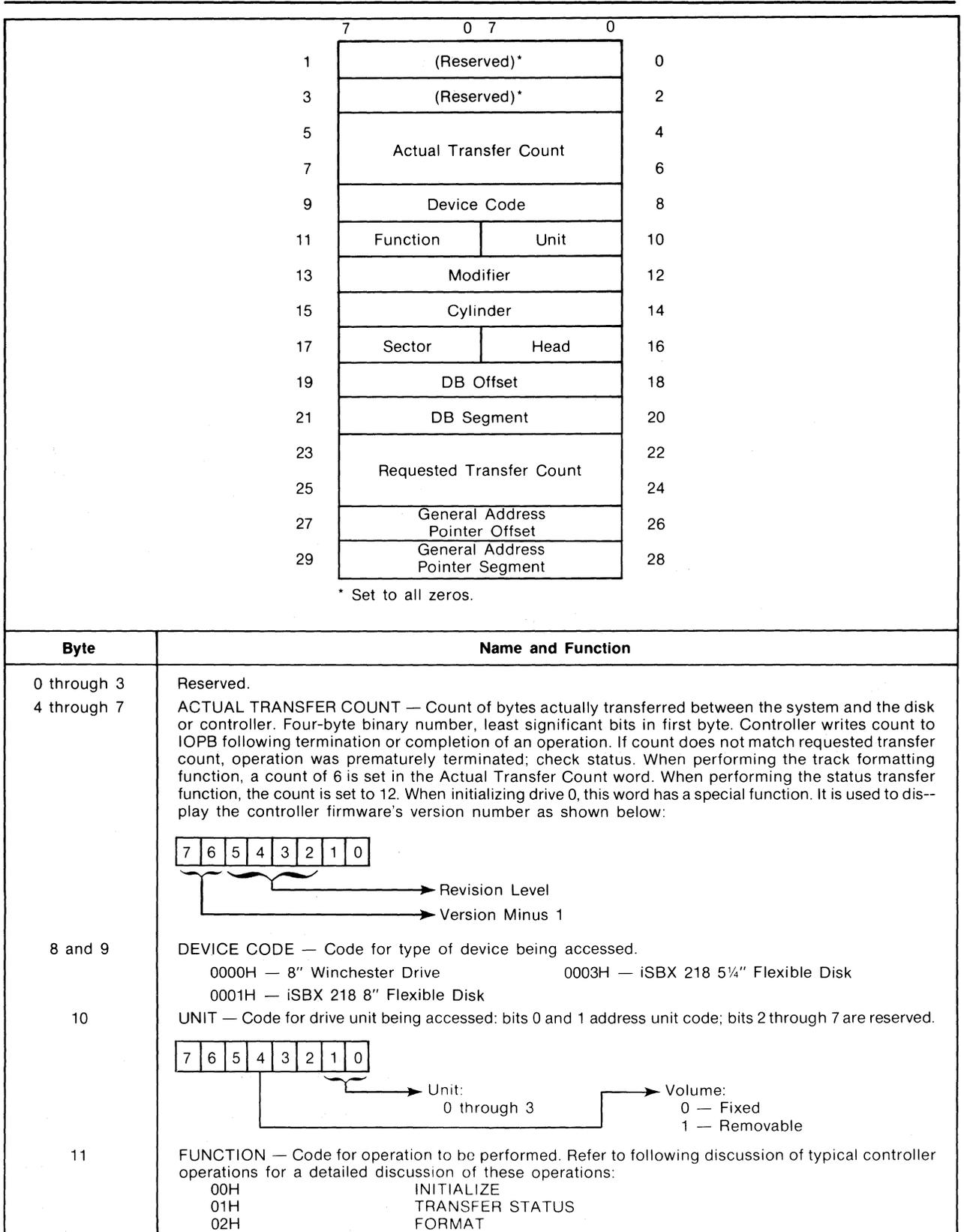
Figure 3-7. I/O Parameter Block Description
