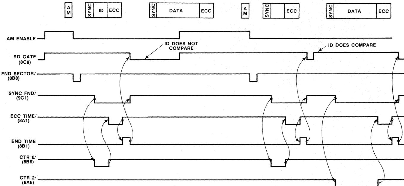
Figure 4-12. Timing Diagram for Read Data Transfer
