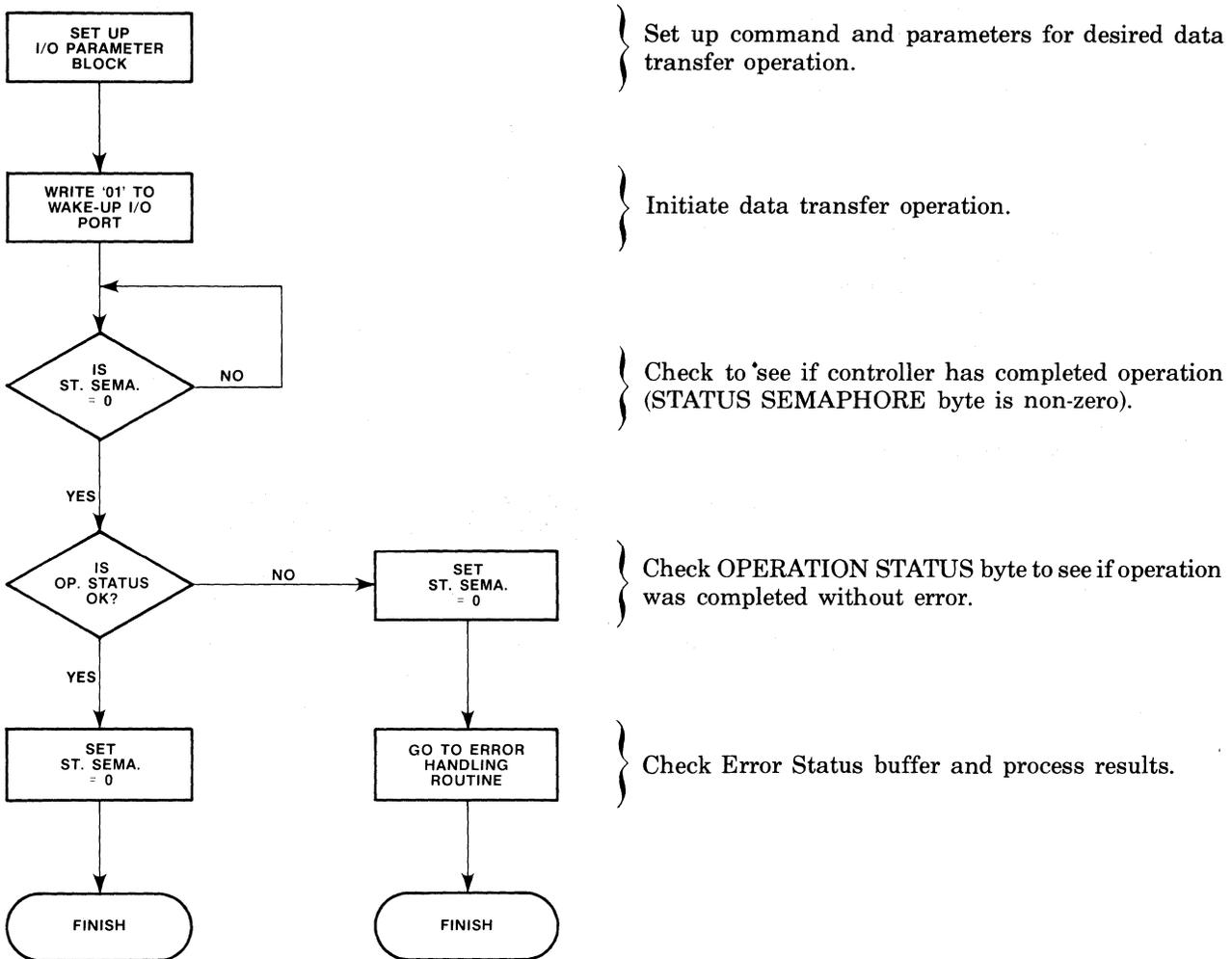
Figure A-1. Flow Chart for Single User Handshake Sequence Without Overlapping Seeks
