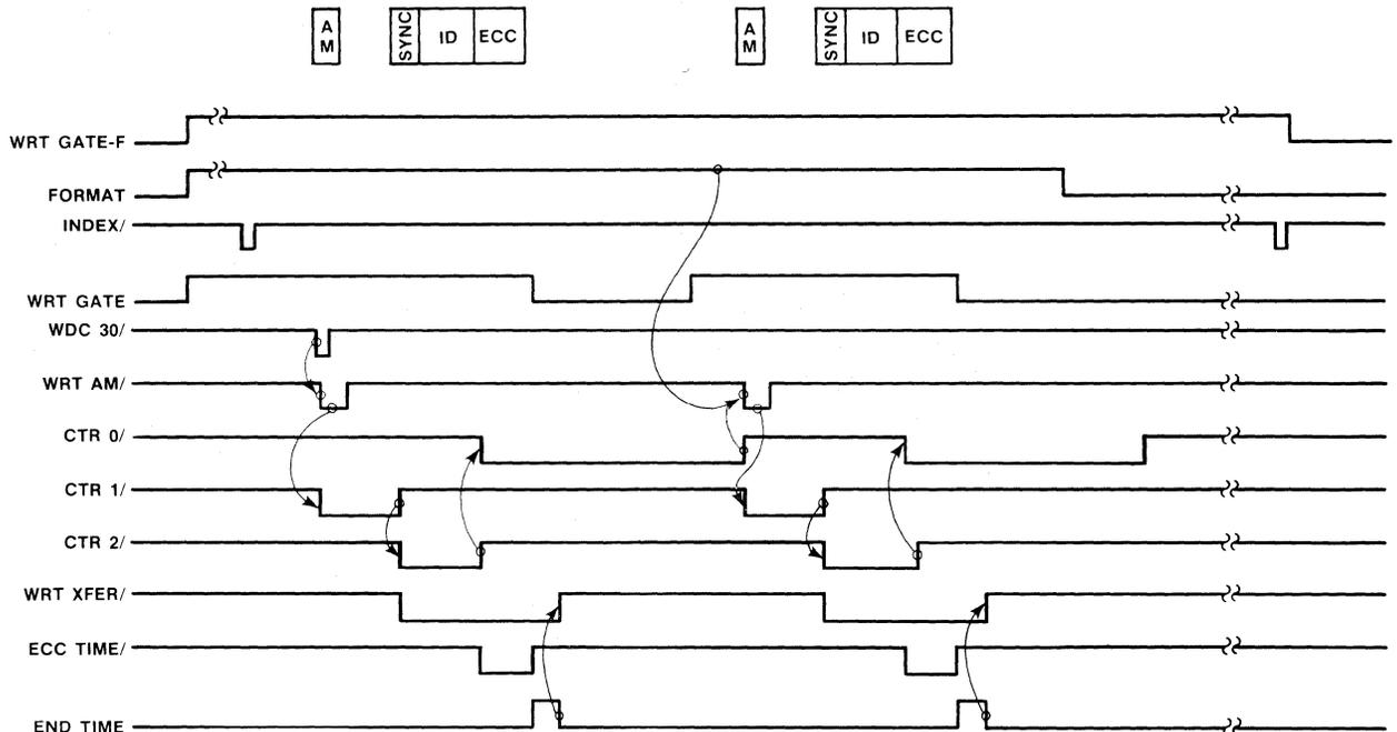
Figure 4-10. Timing Diagram for Disk Formatting Sequence
