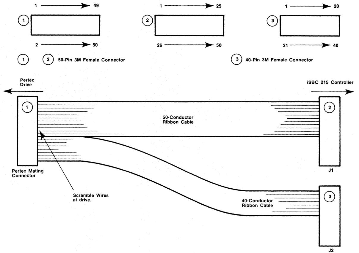
Figure 2-5. Pertec Drive Interconnecting Cable Requirements (Continued)
