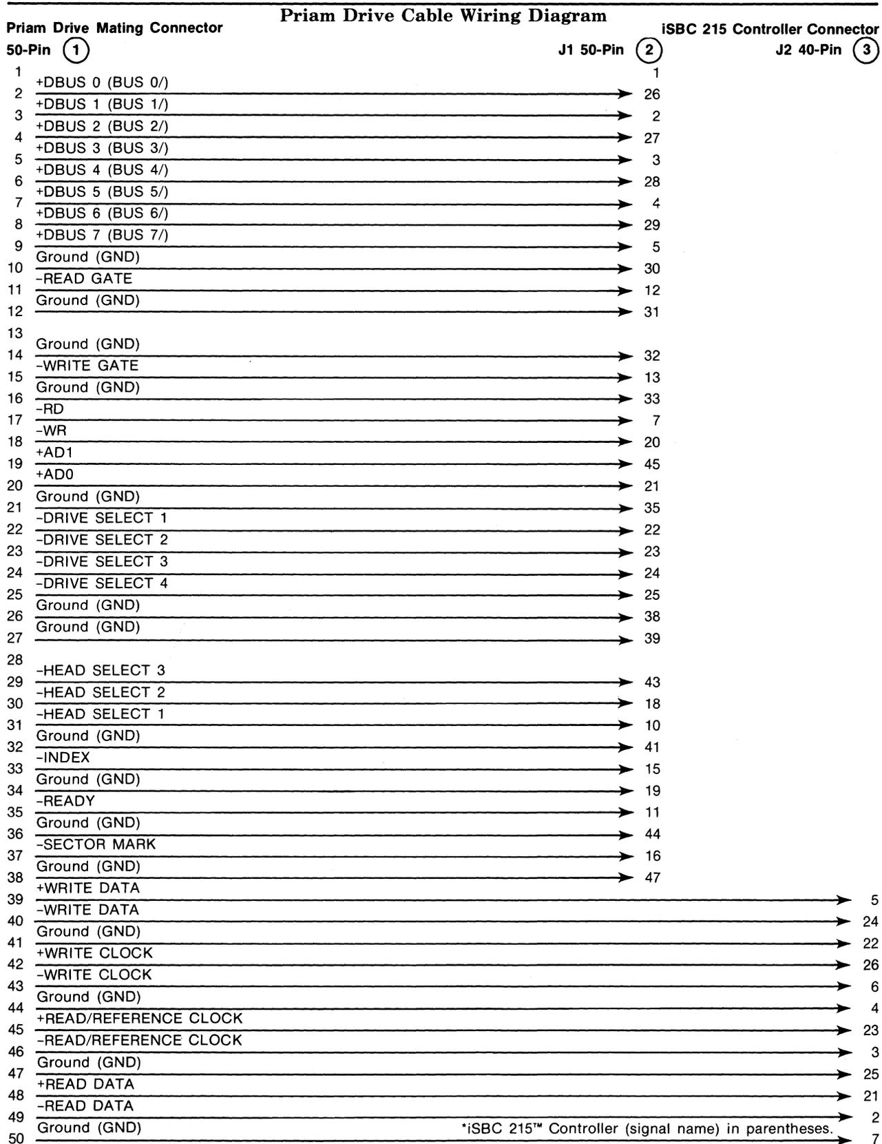
**Figure 2-6. Priam Drive Interconnecting Cable Requirements**
