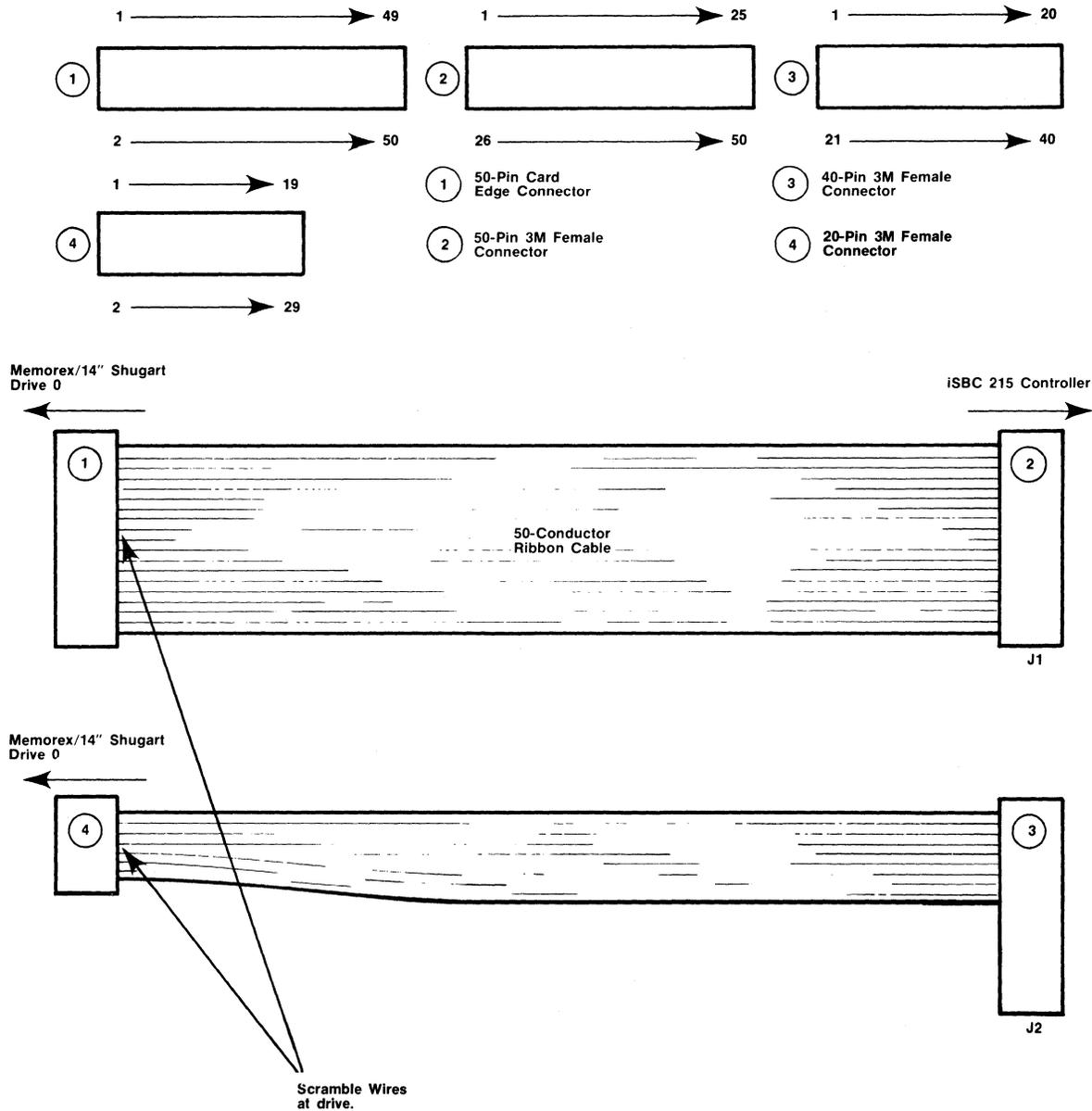
Figure 2-9. Control Data Corporation Drive Interconnecting Cable Requirements
