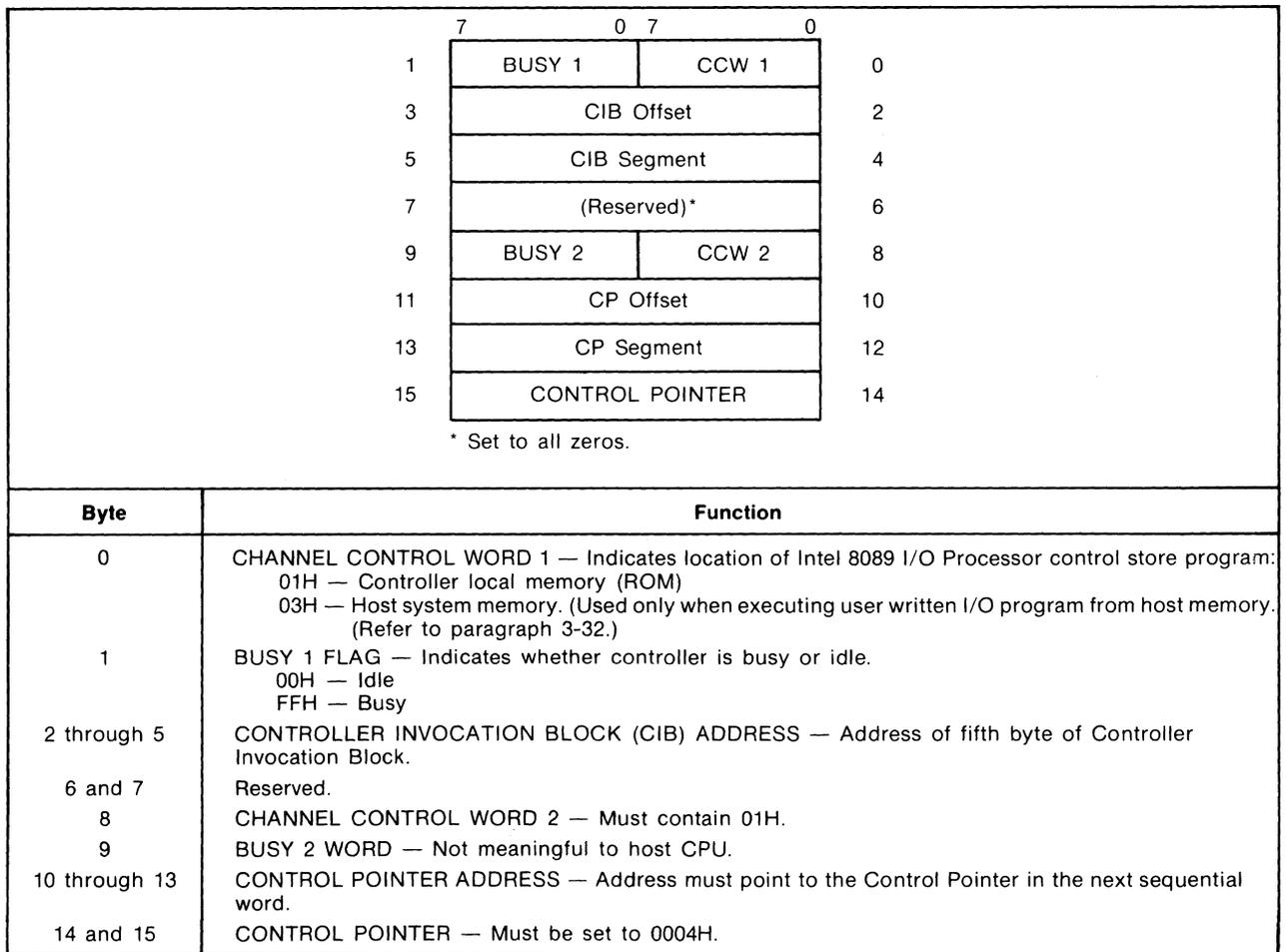
**Figure 3-5. Channel Control Block**
