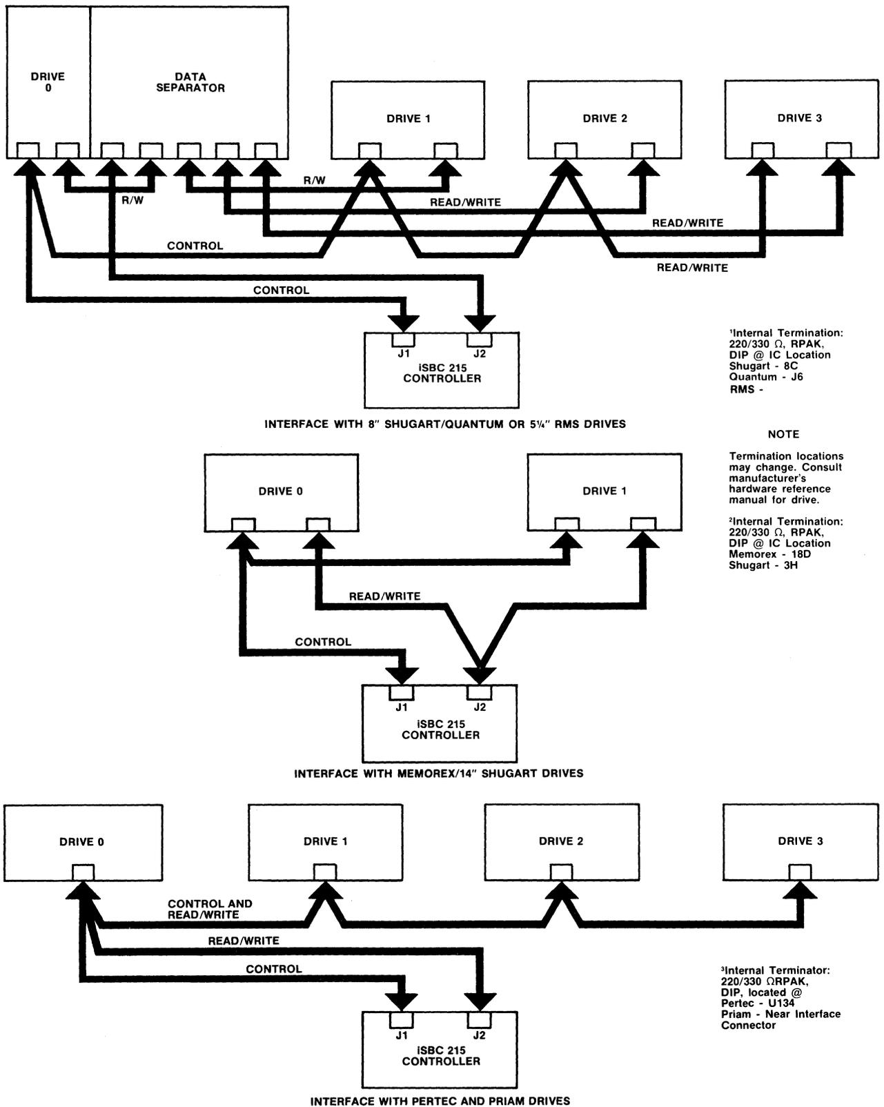
Figure 2-10. Controller to Drive Interfacing
