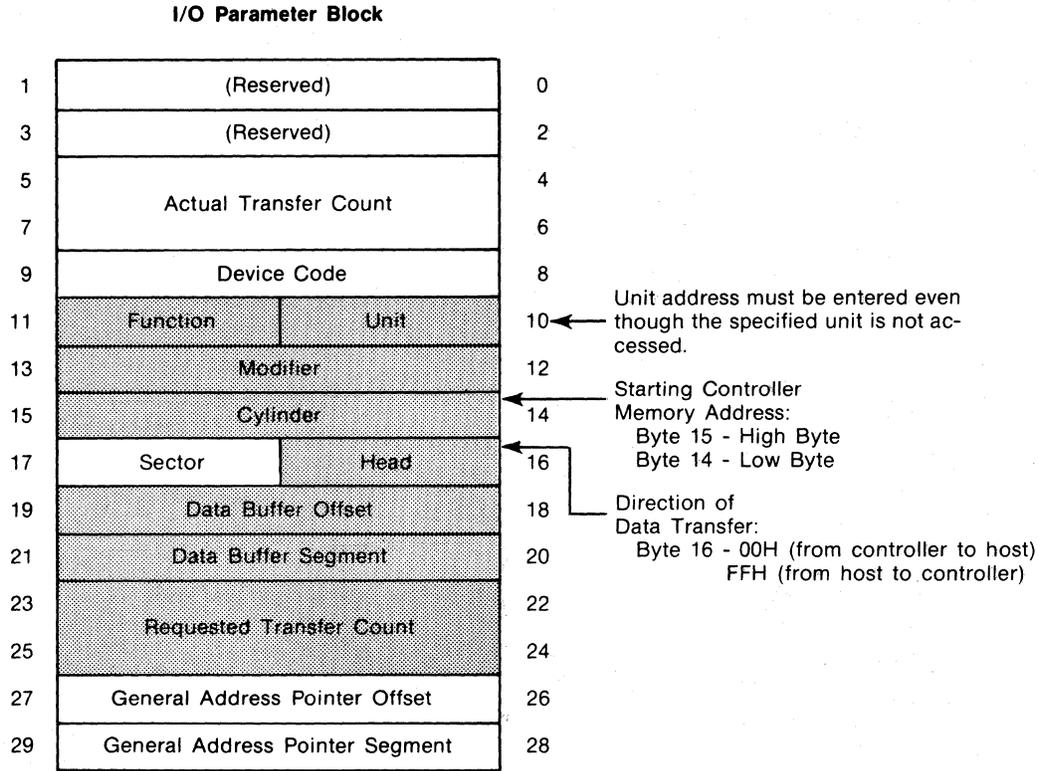
**Figure 3-19. Buffer I/O**
