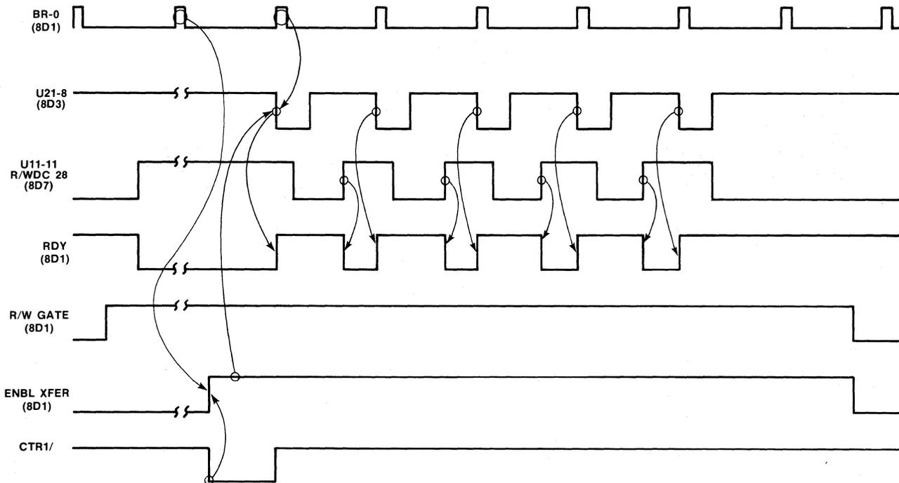
Figure 4-9. Timing Diagram for RDY Signal
