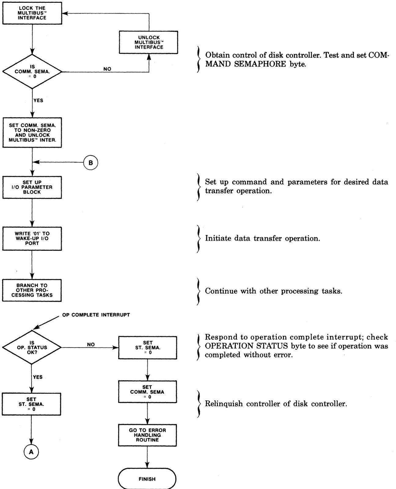
Figure A-3. Flow Chart for Multi-User Handshake Sequence
