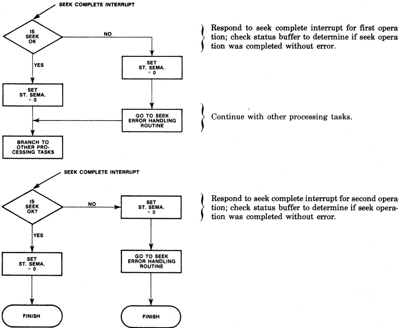
Figure A-2. Flow Chart for Single User Handshake Sequence With Overlapping Seeks (Continued)
