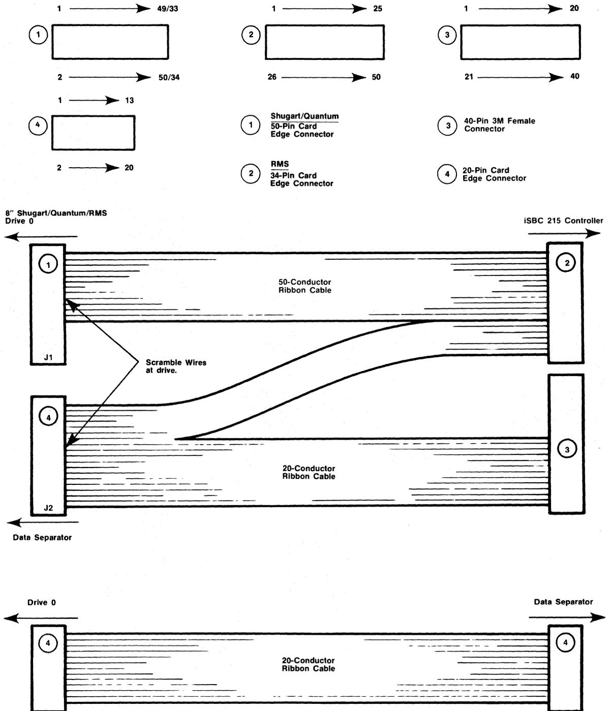
Figure 2-3. 8" Shugart/Quantum Drive Interconnecting Cable Requirements (Continued)
