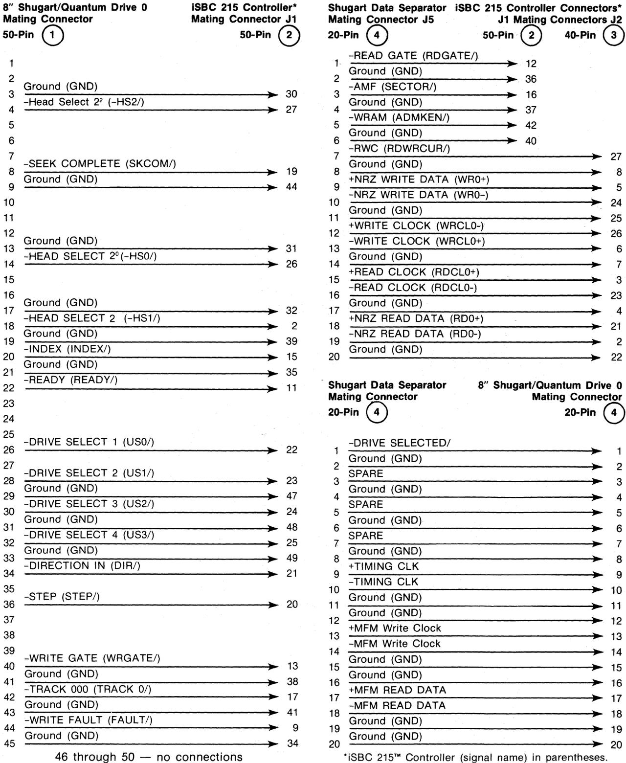
Figure 2-3. 8" Shugart/Quantum Drive Interconnecting Cable Requirements
