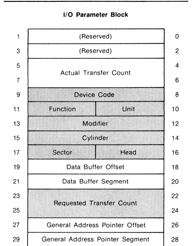
**Figure 3-15. Write Data From Controller Buffer to Disk**
