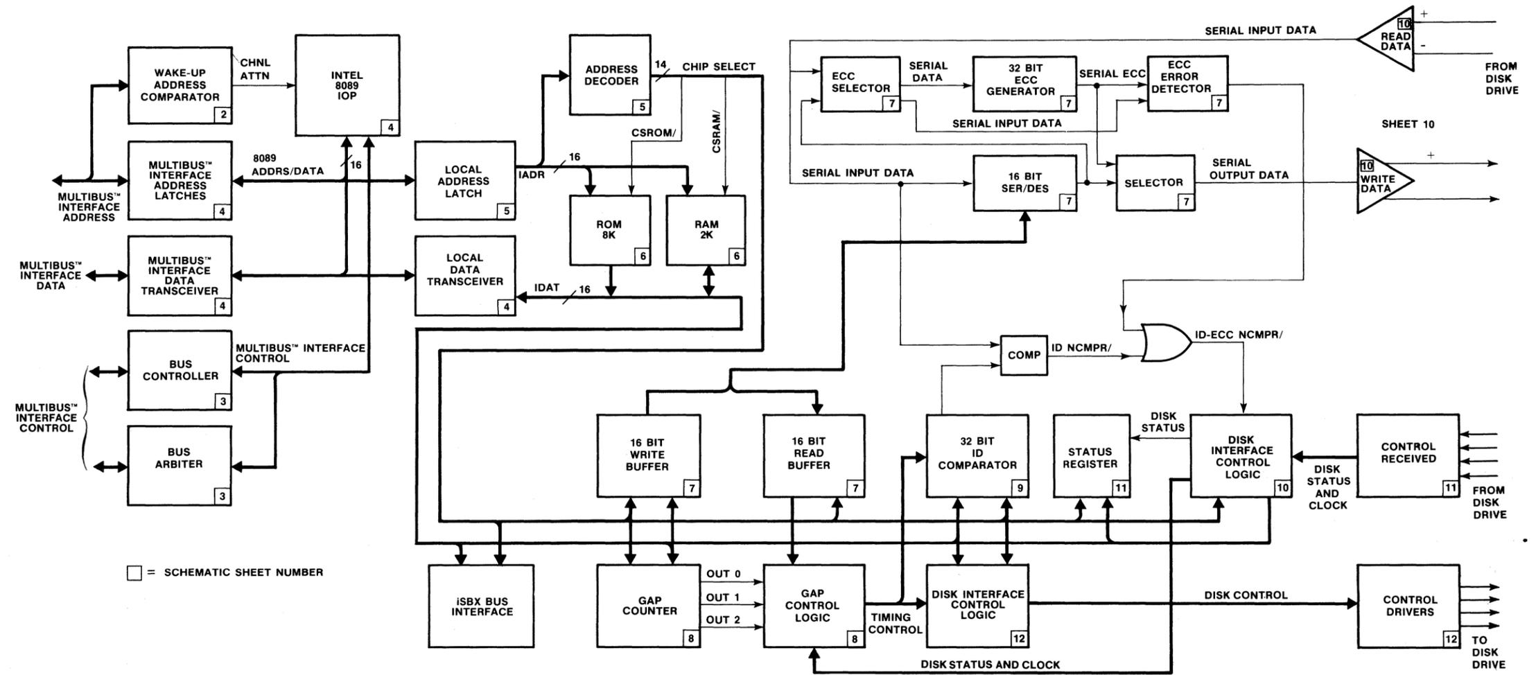
Figure 4-3. iSBC 215™ Controller Functional Block Diagram
