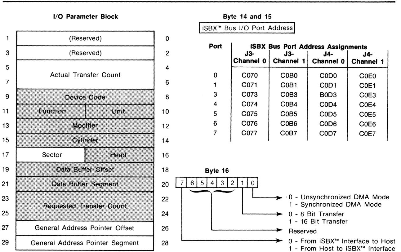
Figure 3-18. I/O Transfers Through iSBX™ Interface
