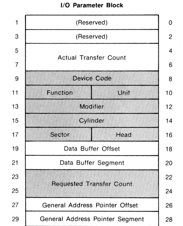
Figure 3-13. Read Data into Controller Buffer and Verify
