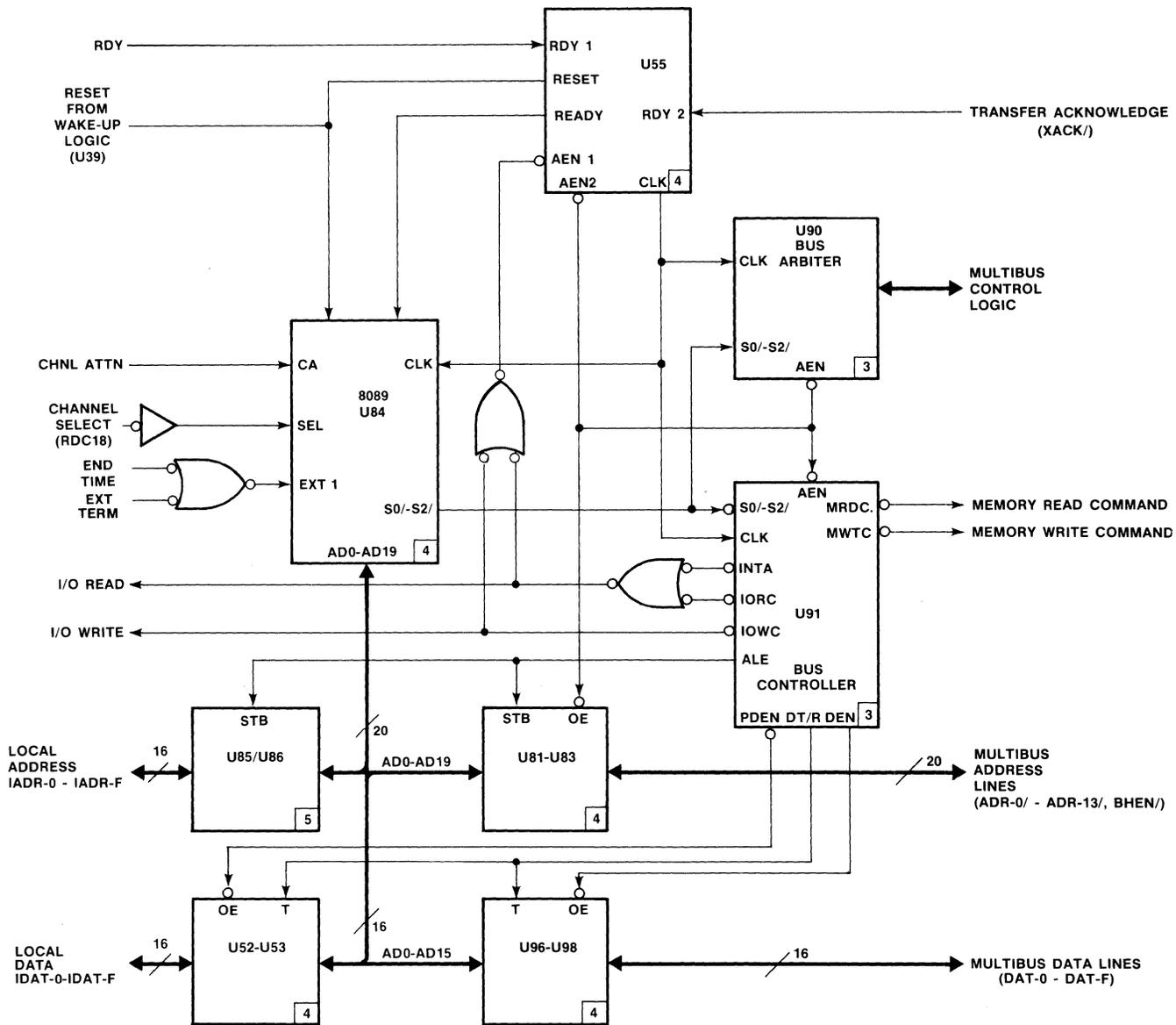
Figure 4-4. Bus Arbiter and Bus Controller Logic
