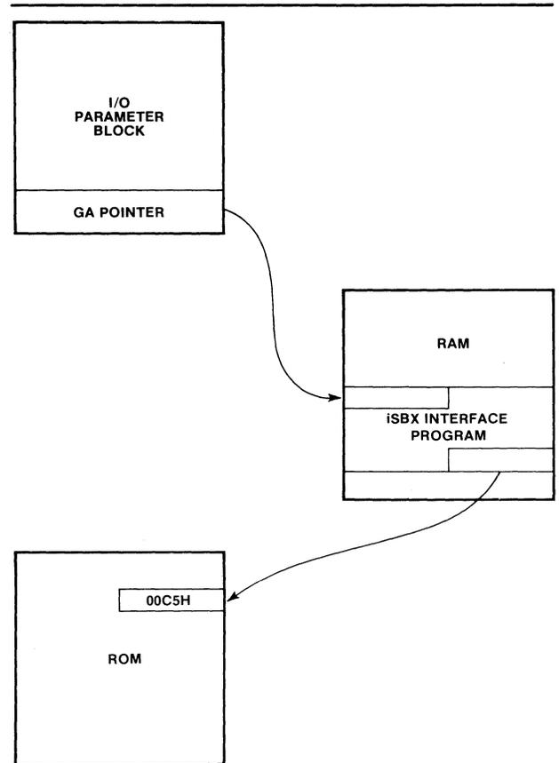
Figure 3-22. Execution of iSBX™ Bus I/O Program From RAM
