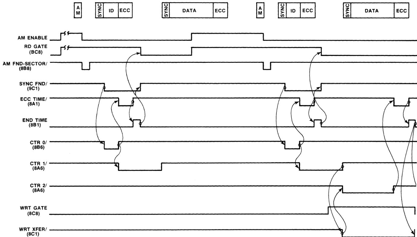
Figure 4-11. Timing Diagram for Write Data
