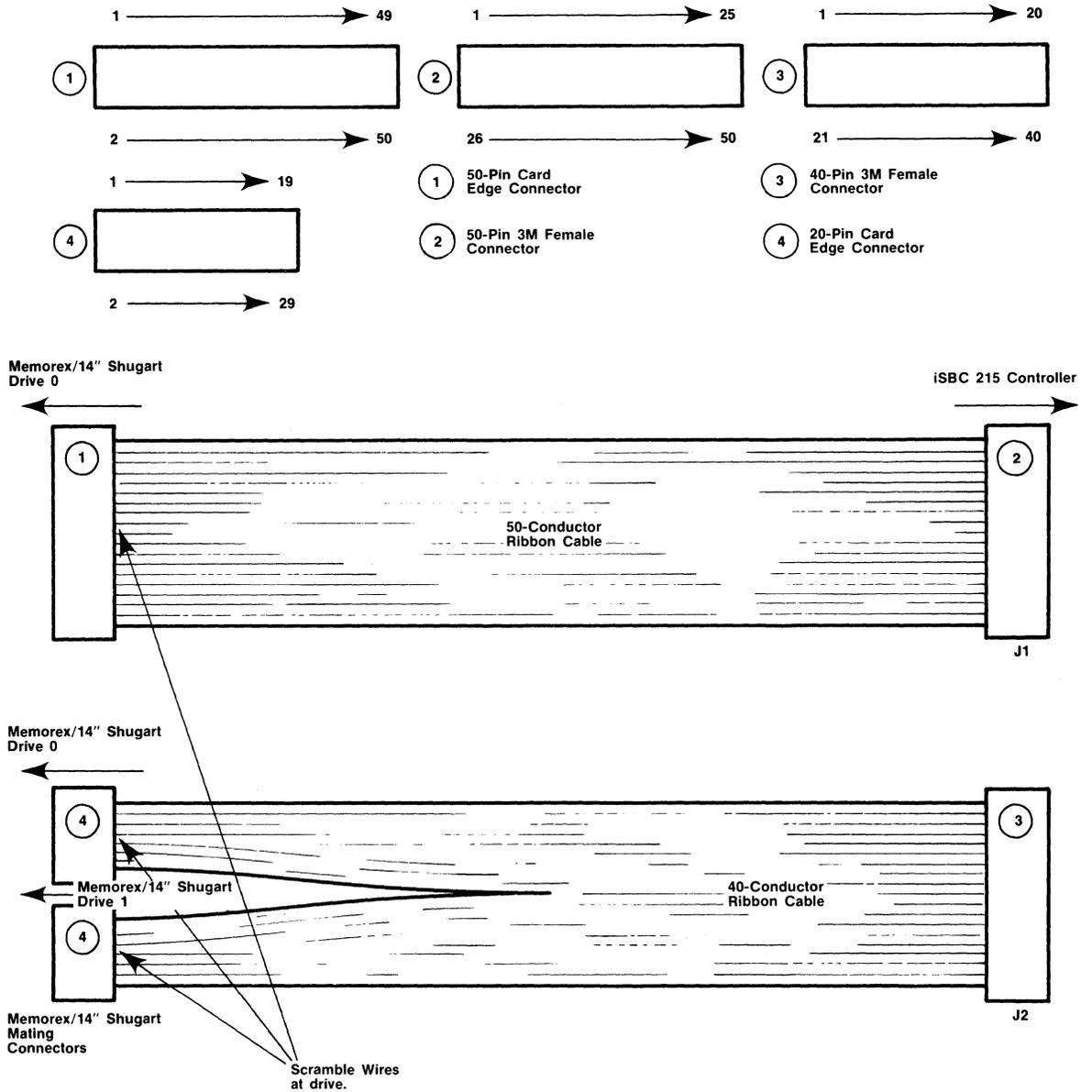
Figure 2-4. Fujitsu 2300/Memorex/14" Shugart Drive Interconnecting Cable Requirements (Continued)
