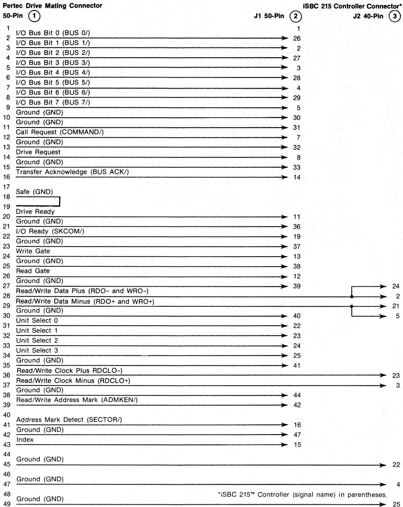
Figure 2-5. Pertec Drive Interconnecting Cable Requirements
