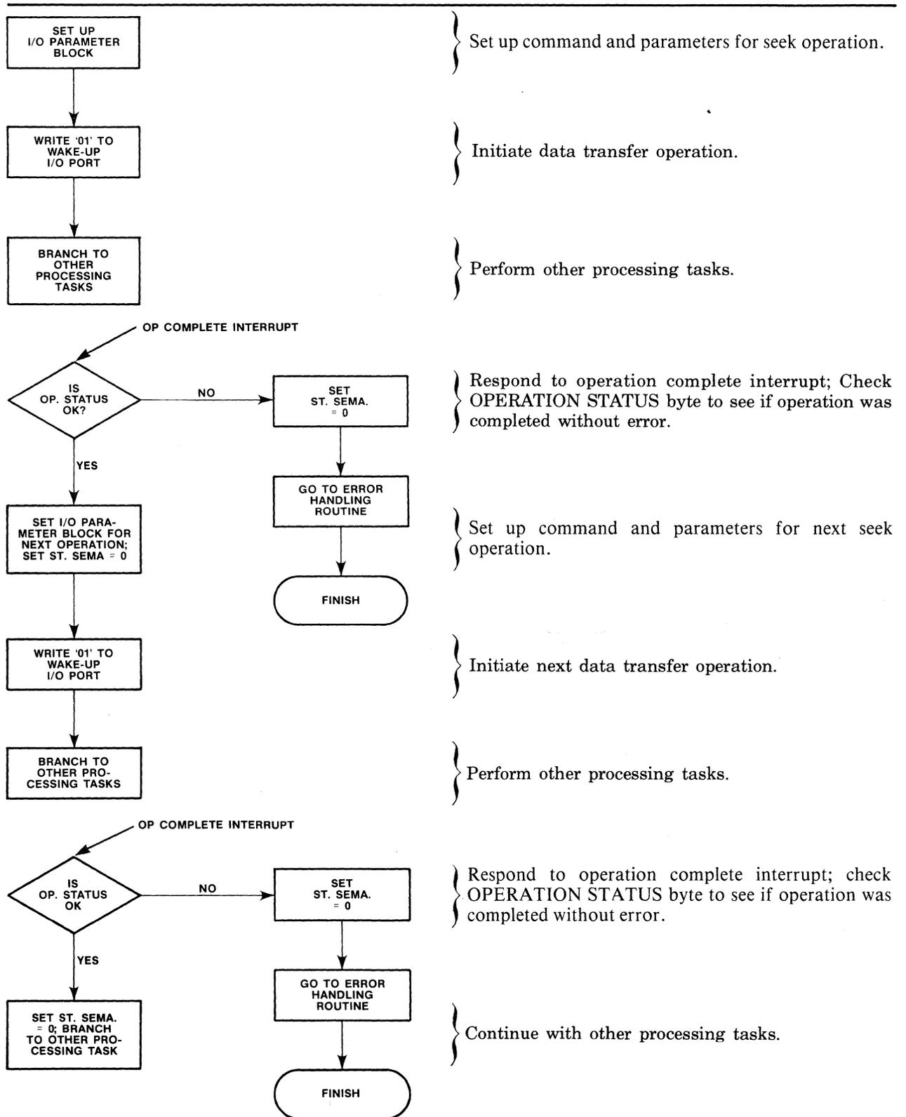
Figure A-2. Flow Chart for Single User Handshake Sequence With Overlapping Seeks
