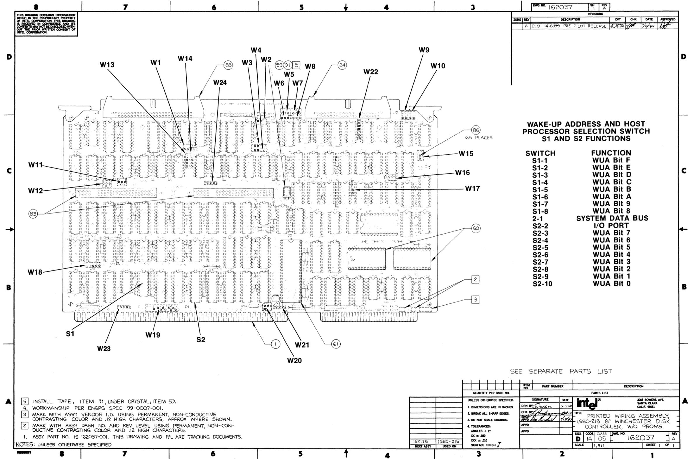
Figure 5-1. iSBC 215™ Controller Jumpers and Switch Locations
