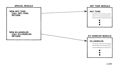
Figure 6-2. Special Module Freezes Entry Points
