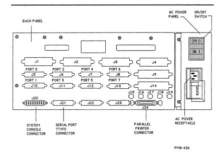
Figure A-2. Eight-User System Serial Port Locations
