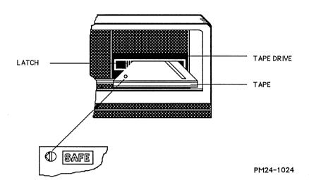
Figure 2-2. Inserting an Archive Tape into a Tape Drive
